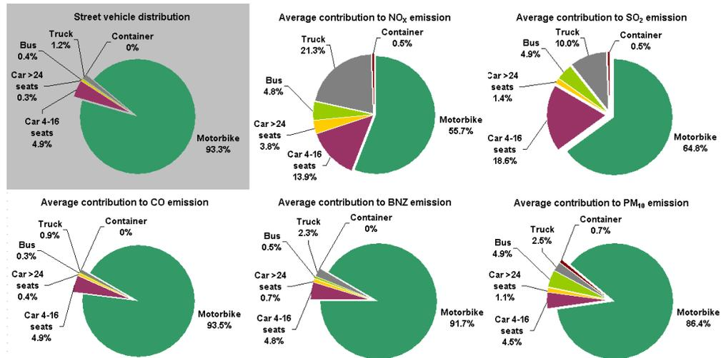
Figure 5. Average contribution (%) to emission of NO<sub>x</sub>, SO<sub>2</sub>, CO, BZN and PM<sub>10</sub> from each vehicle category for five streets in this model evaluation study. The vehicle distribution (%) is shown in the top left chart (source [13]).
