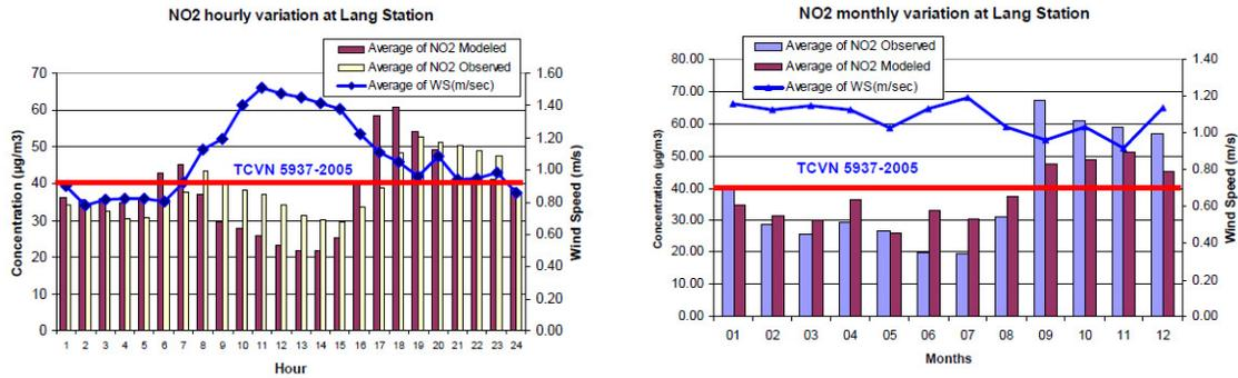
Figure 8. NO<sub>2</sub> modeled vs. NO<sub>2</sub> observed at the Lang Station in 2007 ( $\mu\text{g}/\text{m}^3$ ) by OML model. (source [13]).
