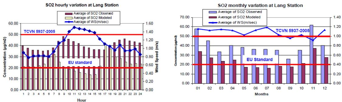
Figure 9. SO<sub>2</sub> modeled vs. SO<sub>2</sub> observed at the Lang Station in 2007 ( $\mu\text{g}/\text{m}^3$ ) by OML model.(source [13]).
