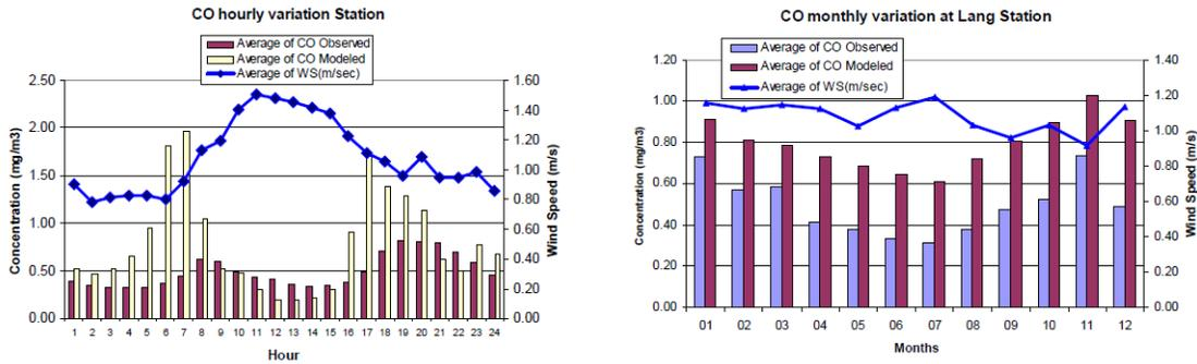
Figure 10. CO modeled vs. CO observed at the Lang Station in 2007 (mg/m<sup>3</sup>) by OML model.(source [13]).
