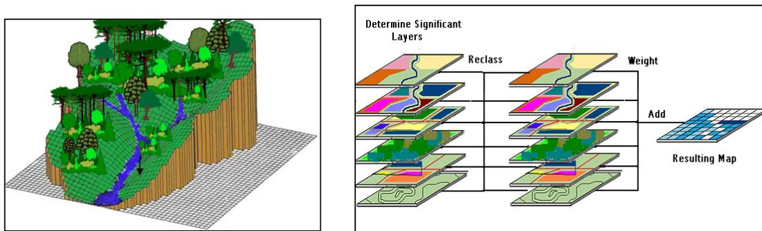
Fig. 4. Simulation in the 3D space and integrating information for mapping flash flood.
