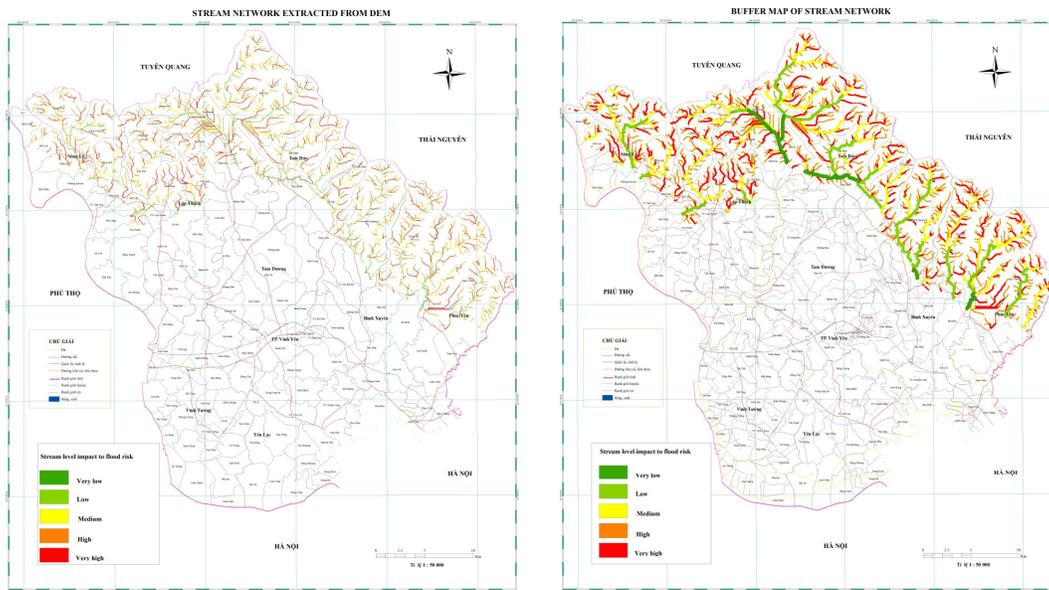
Figure 10. Stream network extracted from DEM (left) and buffers of stream network (right).
