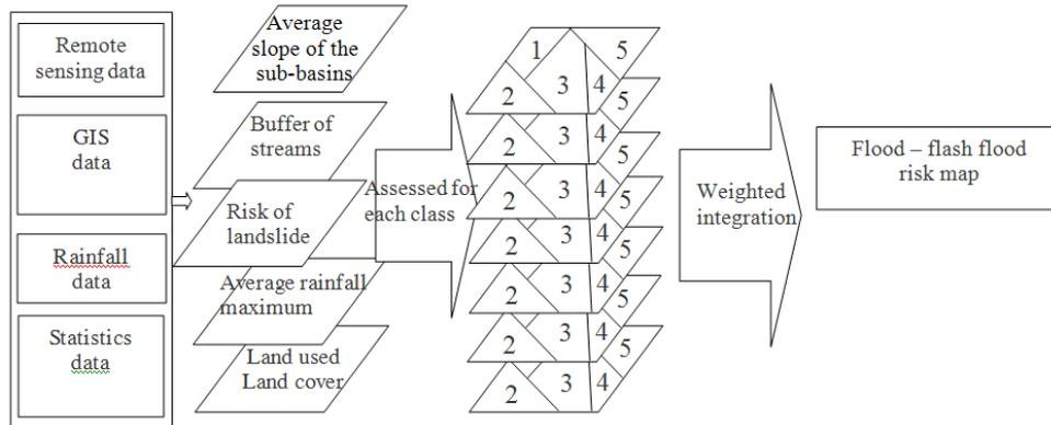
Fig. 5. Weighted model diagram for mapping the risk of muddy - flash flood in Vinh Phuc Province.
