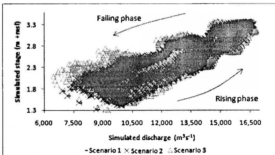
Figure 6. Flow and stage dynamics in the Bassac River (denoted as A, Figure 1.).
