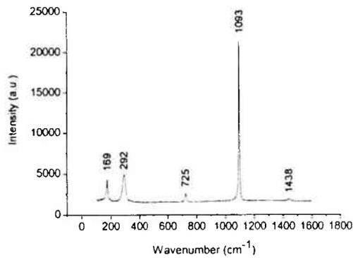
Figure 2b. Raman-spectrum obtained from magnesite in Santa Terezinha emerald.
