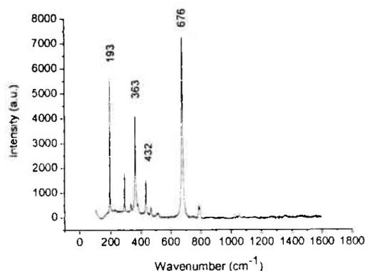
Figure 3b. Raman-spectrum obtained from talc inclusion in Santa Terezinha emerald.
