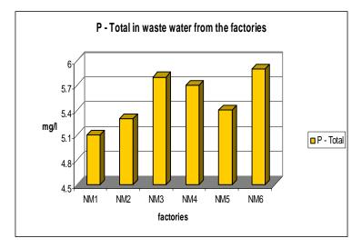
Figure 2. Total phosphorus in waste water of factories.
