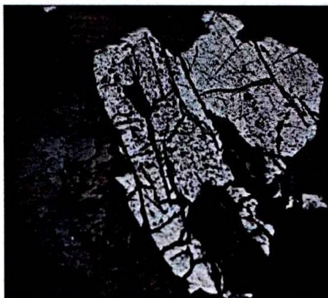
Fig. 3. Semi-euhedral pyrite (sample GL.02).
