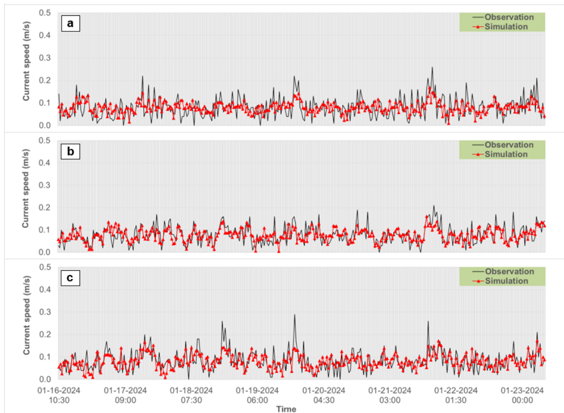
Figure 5. Comparison of current speed at TT2 location by the MIKE model (red) and observations (black) for the (a) surface layer, (b) the middle layer and (c) the bottom layer of the ocean.
