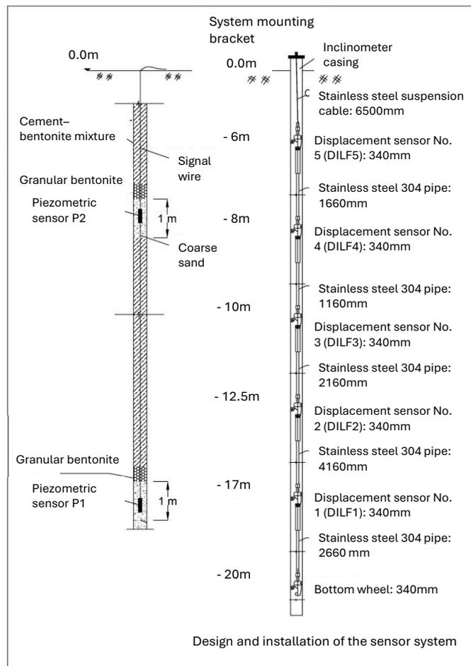
Figure 3. Design and installation of the sensor system.
