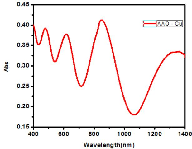
Figure 3. Absorption spectra of the AAO-Cu template.
