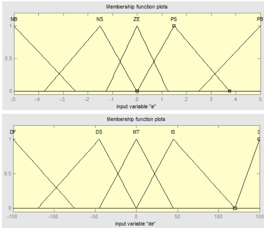
Fig 7. Membership functions of input variables.
