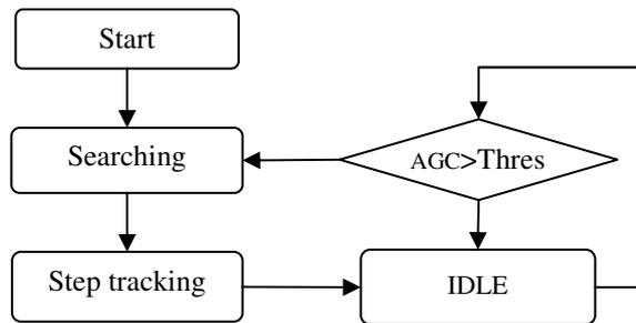
Fig 3. Diagram of step-tracking algorithm.
