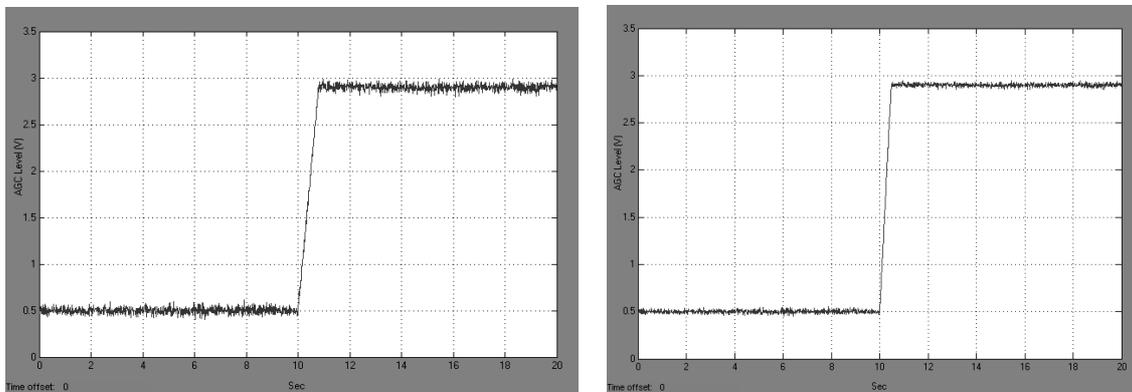
Fig 14. AGC level with PID controller and fuzzy PID controller.
