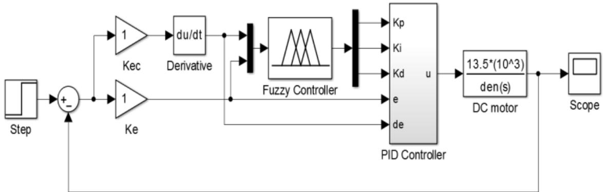
Fig 8. Simulink diagram fuzzy PID controller.
