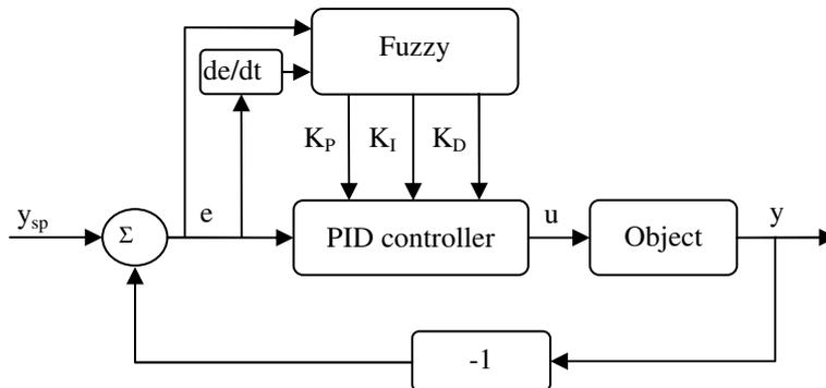
Fig 5. Block diagram of fuzzy PID controller.
