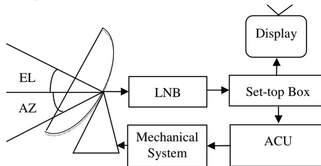
Fig 1. Diagram of the satellite tracking system.
