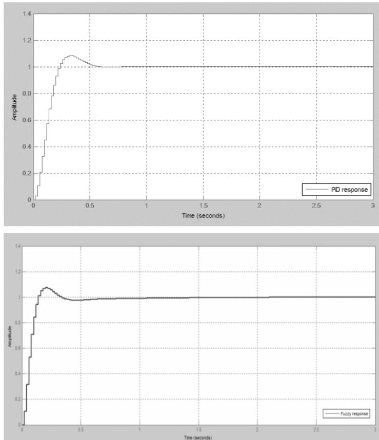
Fig 9. The step response of the PID controller and the fuzzy PID controller.
