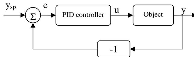
Fig 4. Diagram of PID controller.
