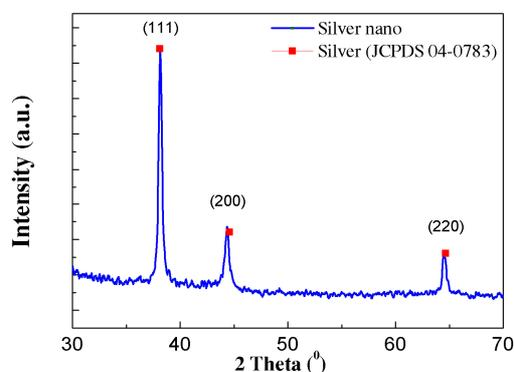
Fig. 2. X-ray diffraction spectra of silver nanoparticles.
