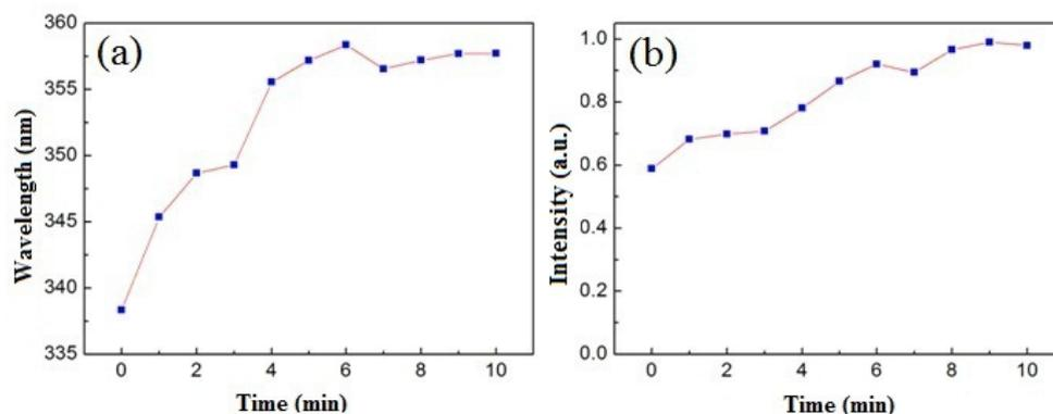
Fig. 7. Dependence of the wavelengths and intensities of absorption peaks of silver nanoparticles solution on the sample boiling time: a) the wavelengths; b) the intensities.
