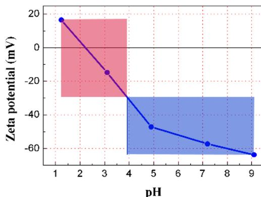
Fig. 5. Zeta potential of silver nanoparticles at different pH values.
