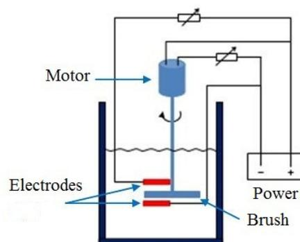
Fig. 1. Diagram of electrochemical system.
