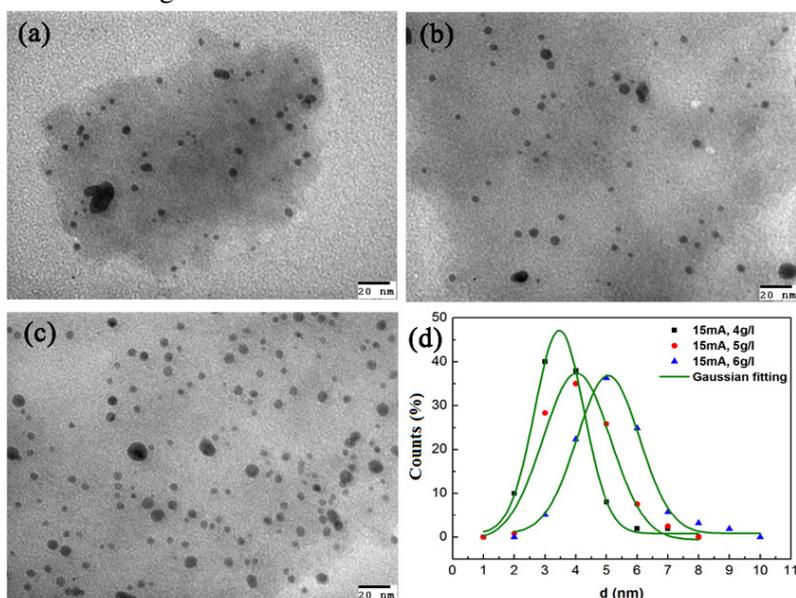
Fig. 3. TEM images of silver nanoparticles ( $I = 15$  mA):  $c = 4$  g/l (a);  $c = 5$  g/l (b);  $c = 6$  g/l (c) and size distribution diagram of silver nanoparticles (d).
