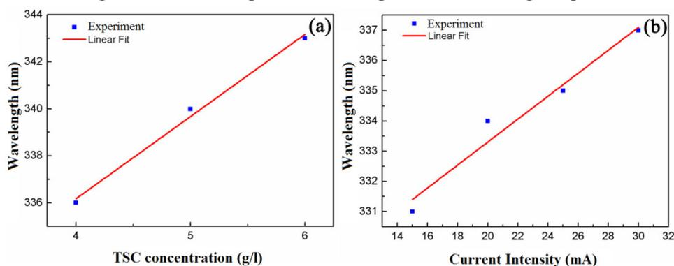
Fig. 6. Dependence of the *wavelength of maximum absorbance* of silver nanoparticles solution on TSC concentration (a) and current density (b).
