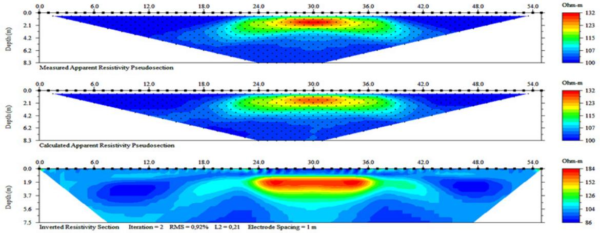
Fig 1d. The experiment result to Wenner array.
