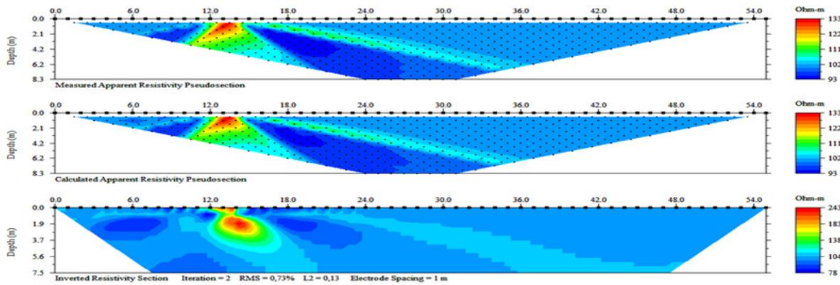
Fig 2d. The experiment result to Wenner array.
