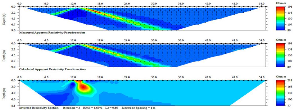
Fig 2c. The experiment result to Dipole-Dipole array.
