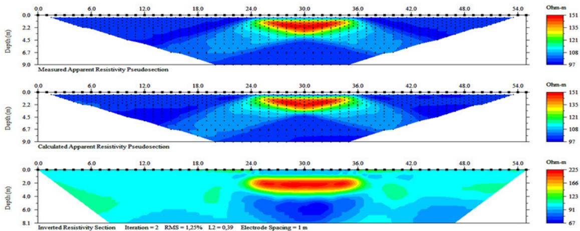
Fig 1c. The experiment result to Dipole-Dipole array.
