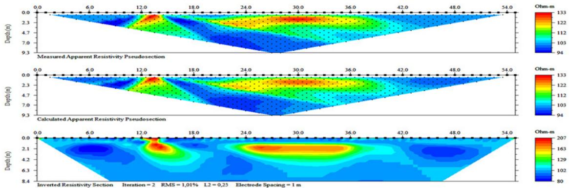
Fig 3d. The experiment result to Wenner array
