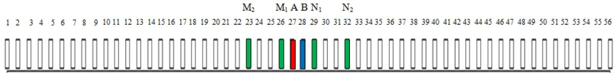
After that, we shall extend AB (in the position 26 and 29), we will get 2 measurement times with 2 MN distances ( $M_1N_1$  in the position 23, 32 and  $M_2N_2$  in the position 14, 41) that could be presented as the following diagram:
