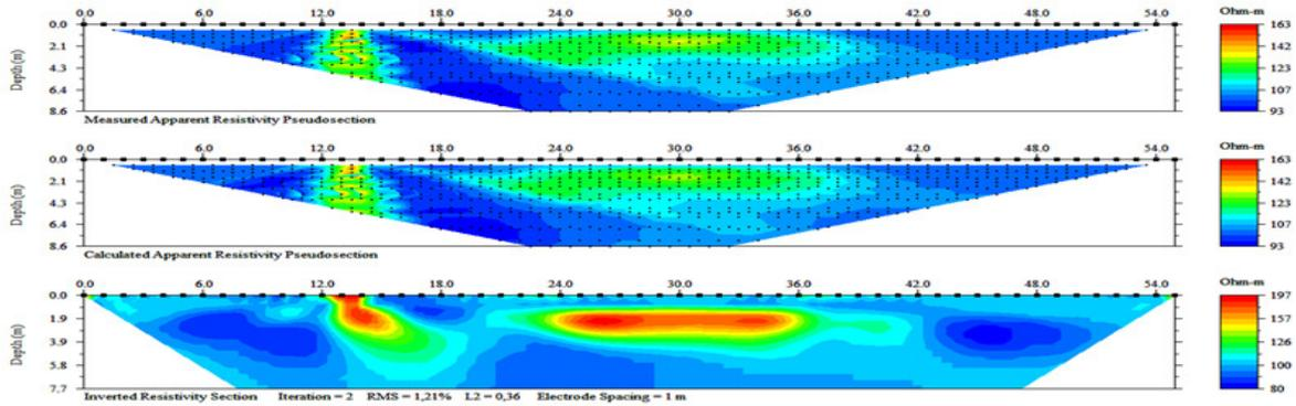
Fig 3b. The experiment result to MC multi-electrode array.
