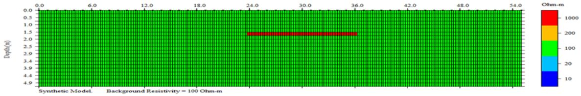
Fig 1a. The experimental model of horizontal seam.
