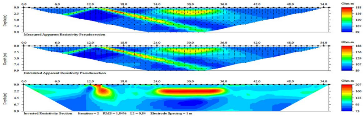
Fig 3c. The experiment result to Dipole-Dipole array.
