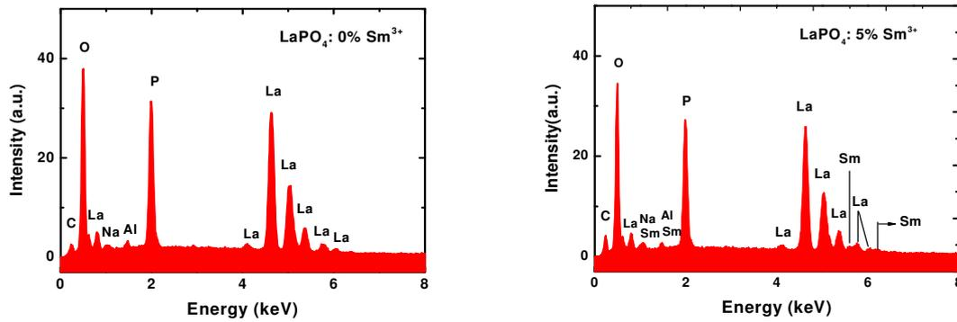
Fig. 7. The EDS spectra of  $\text{LaPO}_4$  and  $\text{LaPO}_4:\text{Sm}^{3+}$  (5 mol%) nanowires prepared at  $220^\circ\text{C}$  for 6 h.
