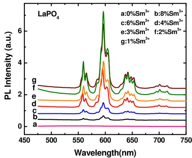
Fig. 9. PL spectra of LaPO<sub>4</sub>: Sm<sup>3+</sup> (0, 1, 2, 3, 4, 6, 8 mol%) under 401 nm excitation wavelength.
