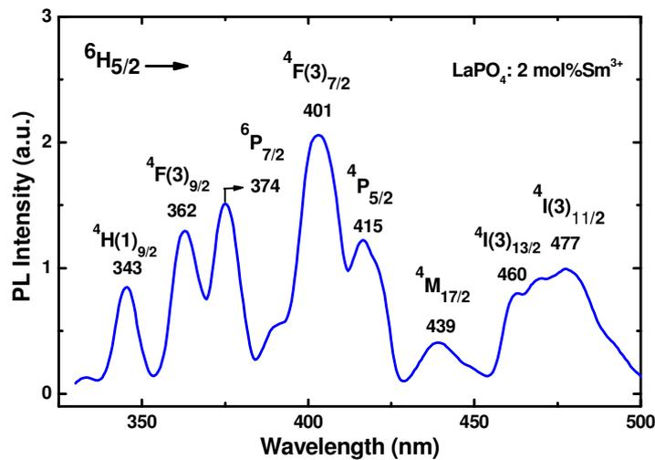
Fig. 11. PLE spectrum monitored at 596 nm of  $\text{LaPO}_4:\text{Sm}^{3+}$  (2 mol%) nanowires.
