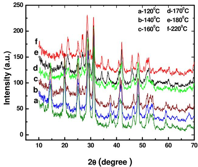
Fig. 2. XRD patterns of  $\text{LaPO}_4$  nanowires prepared at hydrothermal temperatures of 120 – 220°C for 6 h.
