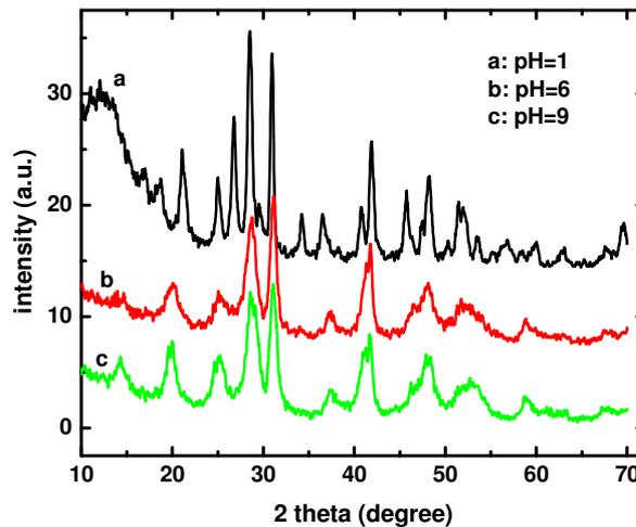
Fig. 4. XRD patterns of the undoped  $\text{LaPO}_4$  nanowires prepared at pH = 1, 6, and 9.
