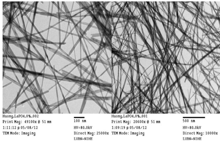
Fig. 1. TEM image of  $\text{LaPO}_4$  nanowires synthesized at 220°C for 6 h.
