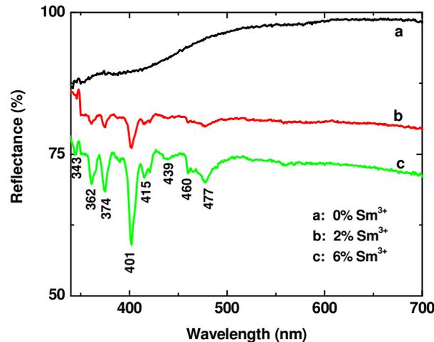
Fig. 12. Diffuse reflection spectra at room temperature of the  $\text{LaPO}_4:\text{Sm}^{3+}$  (0, 2, 6 mol%) nanowires.
