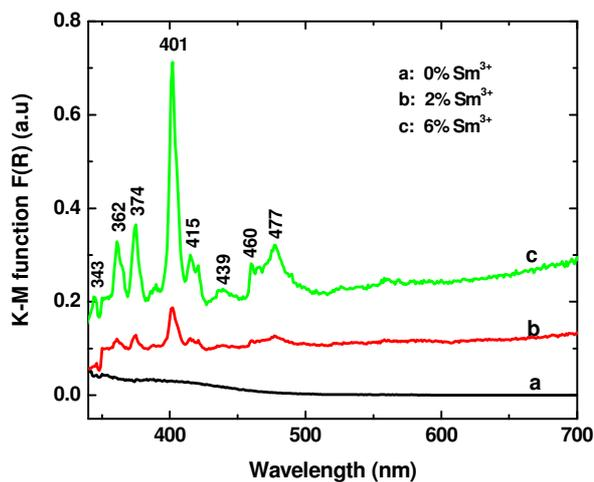
Fig. 13. Plot of Kubelka-Munk function  $F(R)$  proportional to absorption coefficient for the  $\text{LaPO}_4:\text{Sm}^{3+}$  (0, 2, 6 mol%) nanowires.
