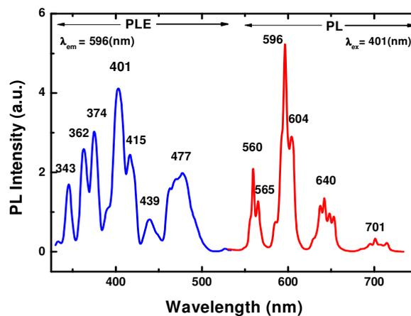
Fig. 8. Typical PL and PLE spectra of  $\text{LaPO}_4:\text{Sm}^{3+}$  (2 mol %) nanowires.
