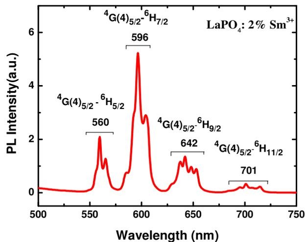
Fig. 10. PL spectrum of LaPO<sub>4</sub>: Sm<sup>3+</sup> (2 mol%) nanowires under 403 nm excitation wavelength.
