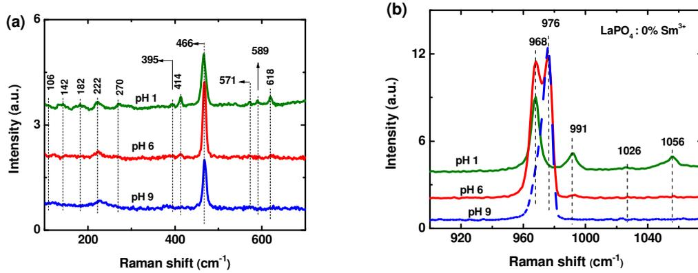
Fig. 6. Room temperature Raman spectra of the  $\text{LaPO}_4$  nanopowders prepared at pH = 1, 6, and 9 in various wavenumber region (a) from  $100 \text{ cm}^{-1}$  to  $700 \text{ cm}^{-1}$  and (b) from  $900 \text{ cm}^{-1}$  to  $1080 \text{ cm}^{-1}$ .
