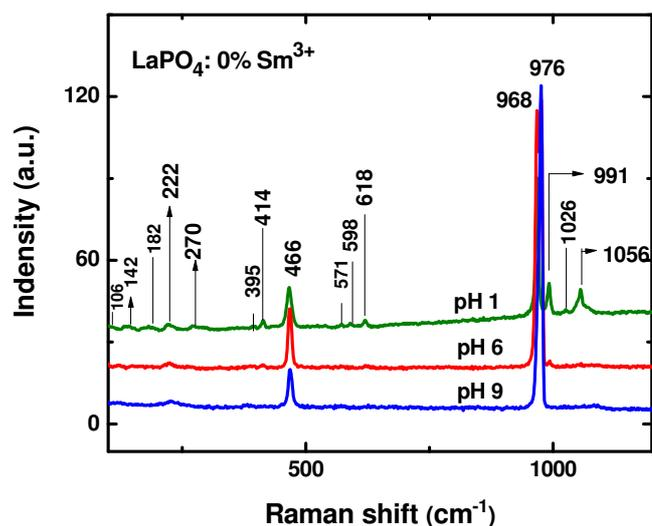
Fig. 5. Room temperature Raman spectra of  $\text{LaPO}_4$  nanopowders prepared at pH = 1, 6, and 9.
