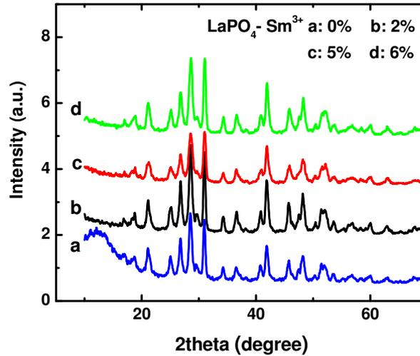
Fig. 3. XRD patterns of  $\text{LaPO}_4:\text{Sm}^{3+}$  (0, 2, 5, and 6 mol%) nanowires prepared at 220 °C for 6 h.
