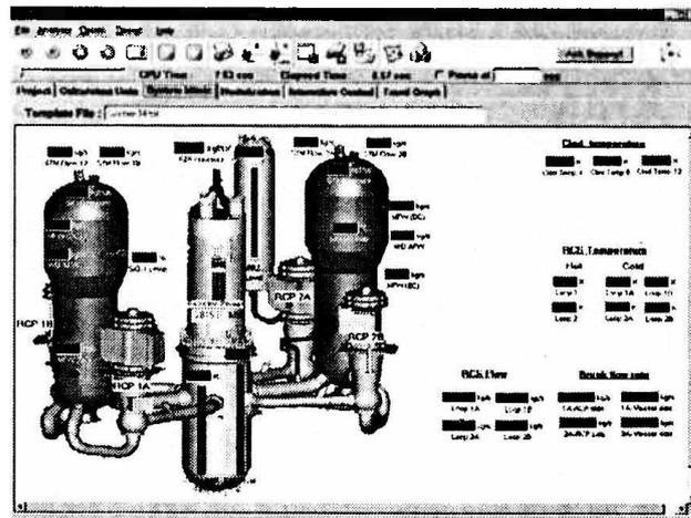
Fig. 1. Graphical simulation of a typical Western PWR (Mimic functions) (figure from [5]).
