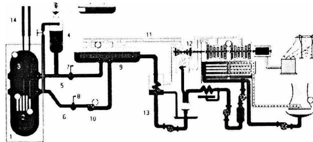
Fig. 3. Overview of the thermal hydraulic system of a typical VVER reactor (horizontal steam generator).
