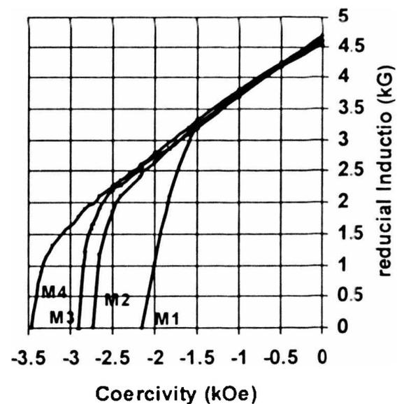
Fig. 1. Demagnetizing curves of anisotropic samples M1- M4.
