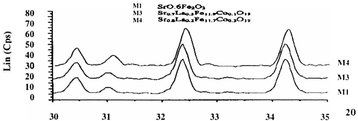
Fig. 3. X-ray diffraction patterns of the samples M1, M3 and M4 sintered at 1260°C/2h.
