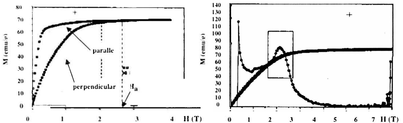
Fig. 2.  $M(H)$  curve (left) and  $\frac{d^2 M(H)}{dH^2}$  curve (right) of sample M4 sintered at 1260°C/2h.
