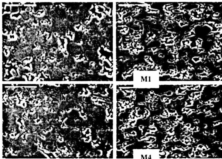
Fig. 5. SEM Images of anisotropic bulk samples M1, M4 perpendicular (left) and parallel (right) to the preferred magnetizing direction (bright line is 10 μm).
