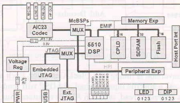
Fig. 1. Inside architecture of TMS320VC5510 DSK.
