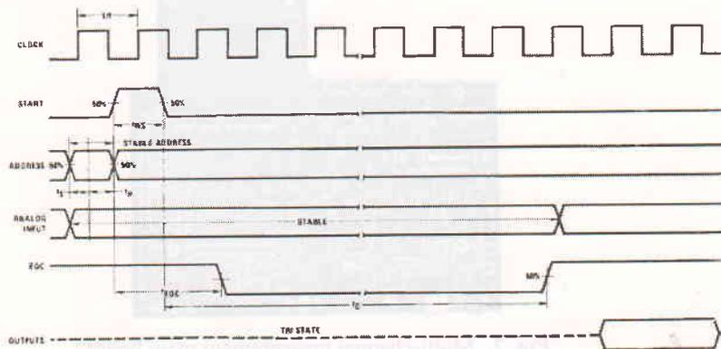
Fig. 5. ADC Timing Diagram.
