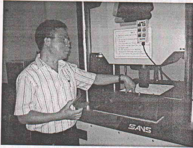
Fig. 1. Bending test for 3-phase composite plate.
