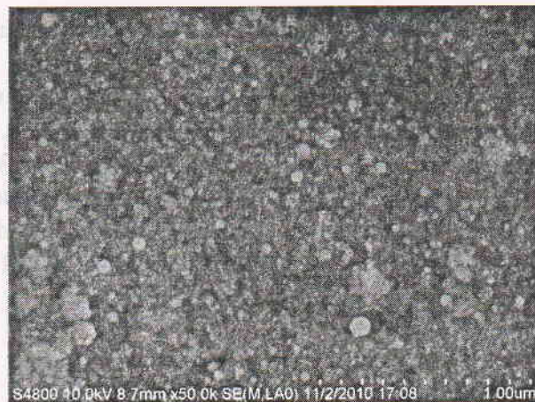
Fig. 2. Scanning electron micrographs of SERS substrates.
