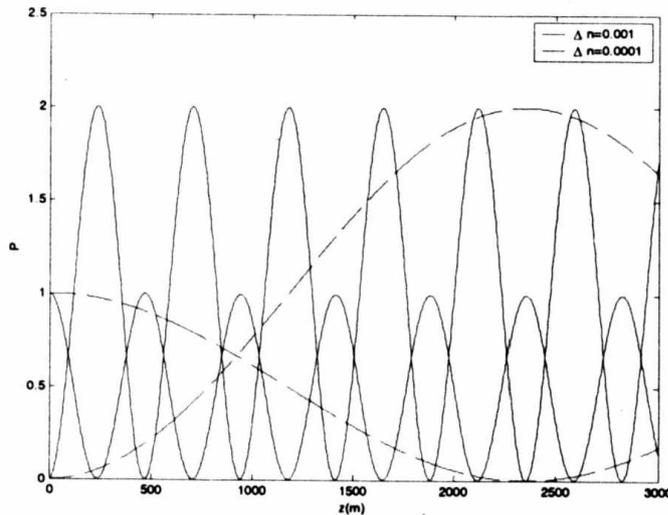
Fig.2. The diagram allows to determine the dependence of  $L_0$  on  $\Delta n$
