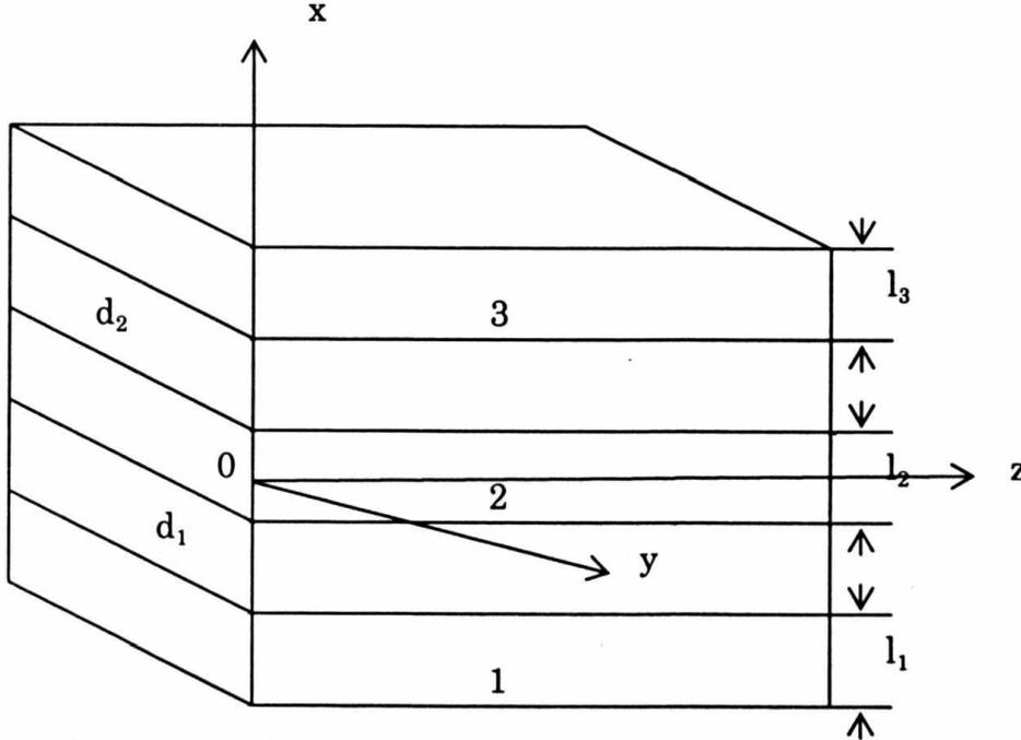
Fig. 1 . Model of three monomode plan wave guides.
