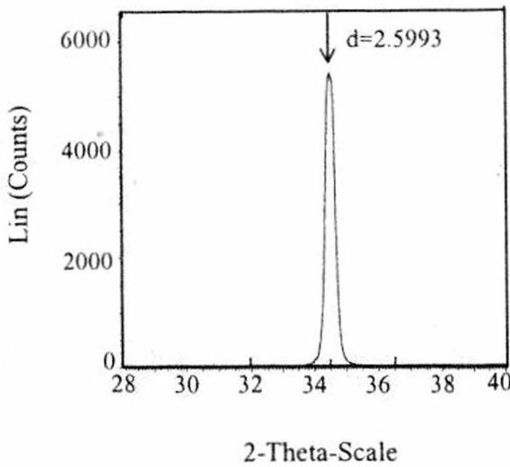
Fig. 2. X-ray diffraction pattern of a  $ZnO:Al$  film deposited on glass substrate
