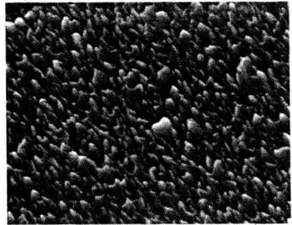
Fig. 3. SEM of  $ZnO:Al$  film deposited on glass substrate at *r.f* power 100 W and argon pressure  $8.8 \times 10^{-3}$  Torr
