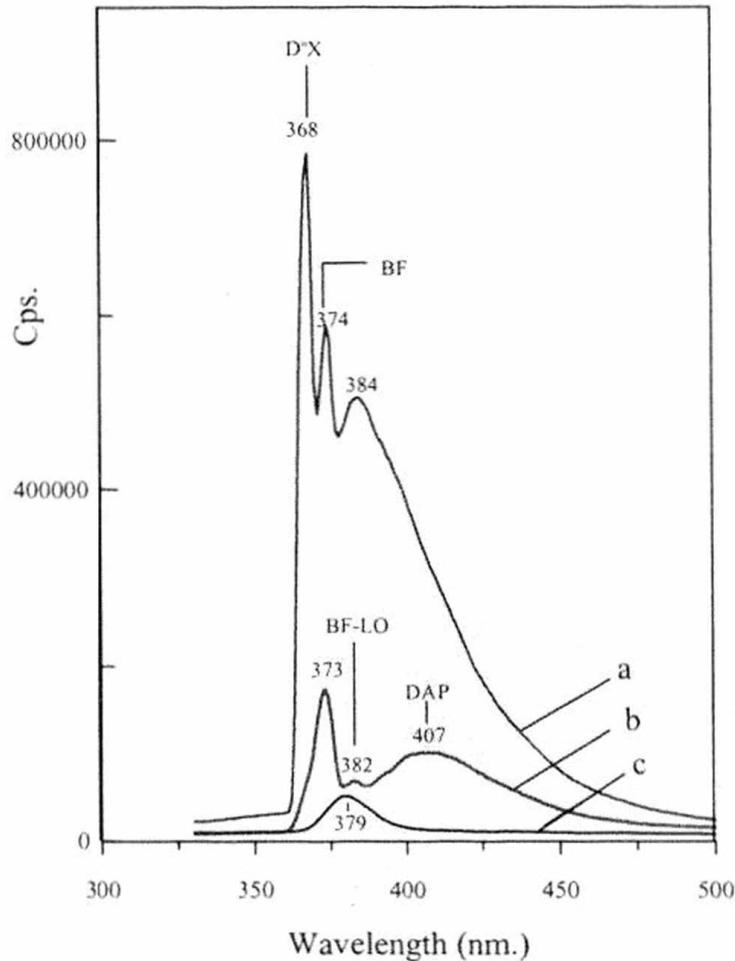
*Fig. 6.* PL spectra of ZnO:Al films with excitation wavelength 300 nm at different temperatures:
