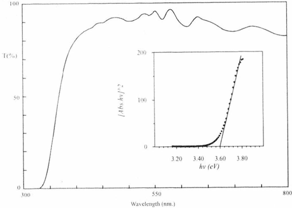
Fig. 5. Optical transmittance of a ZnO:Al film deposited on glass substrate at r.f power 350 W and argon pressure  $8.8 \times 10^{-3}$  Torr.
