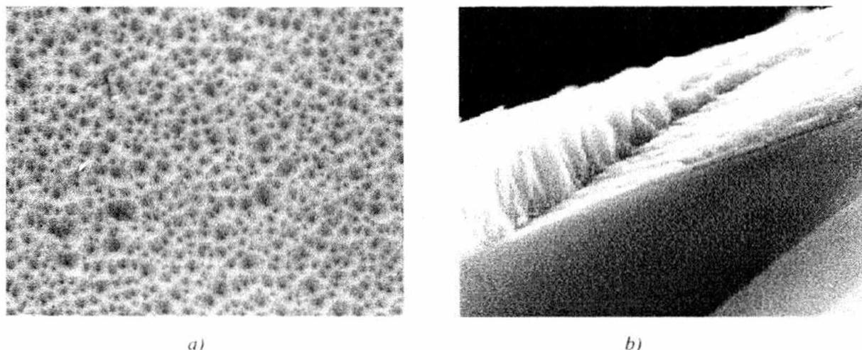
Fig. 1. SEM surface (a) and cross - section (b) micrographs of a ZnO:Al film on glass substrate at *r.f* power 350 W and argon pressure  $8.8 \times 10^{-3}$  Torr
