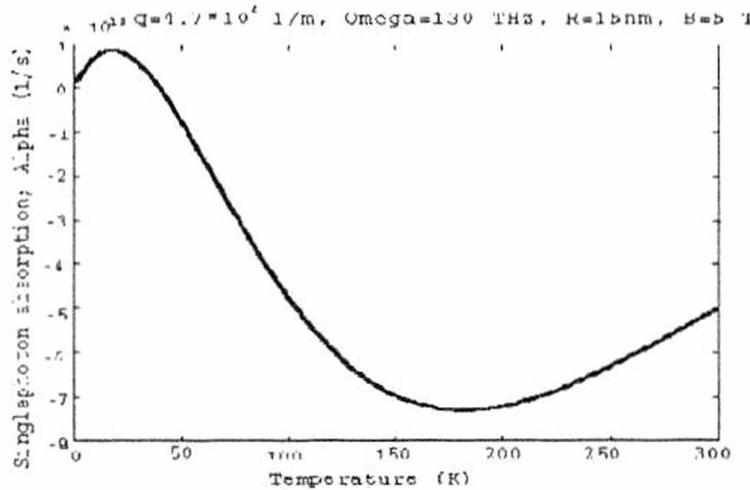
Figure 3. Dependence of the rate of phonons excitations on temperature in the case of singlephoton absorption process;  $\Omega = 130Thz$ ,  $R = 15nm$ ,  $q = 4.710^6m^{-1}$ ,  $B = 5T$
