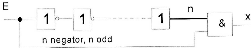
Fig. 2. Delay caused by the negator.
