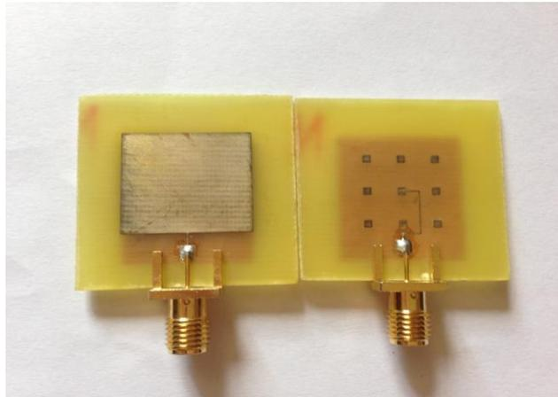
a) A microstrip antenna and a meta-antenna.
