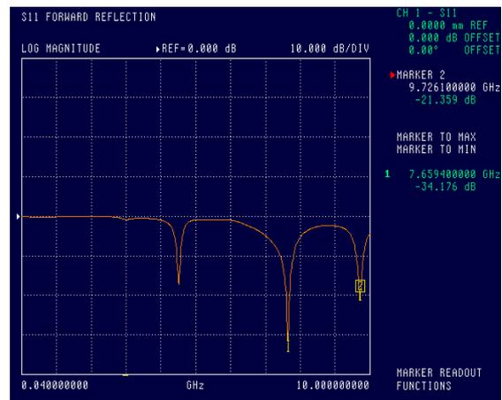
c) Resonance characteristic of the optimized meta-material antenna.
