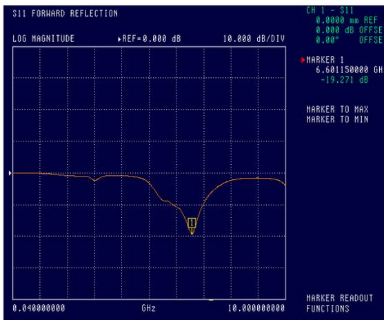
b) Resonance characteristic of the microstrip antenna.
