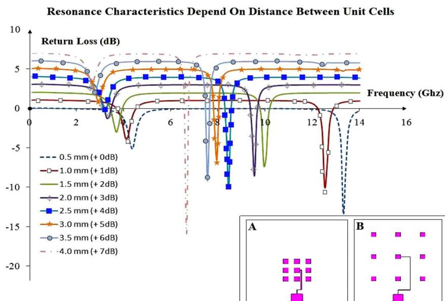
Figure 4. Resonance characteristics depends on distance between unit cells
