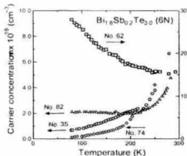
Fig.4. Temperature dependence of the carrier concentration  $n$  of  $\text{Bi}_{1.8}\text{Sb}_{0.2}\text{Te}_3$  sample.
