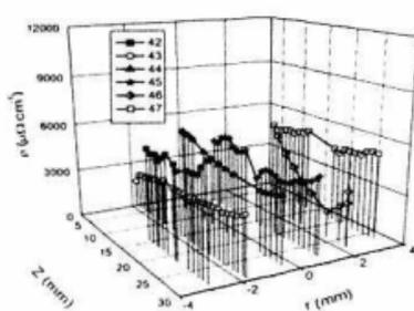
**Fig.3b.** Position dependence of the electrical resistivity for samples No. 42 to No. 47.
