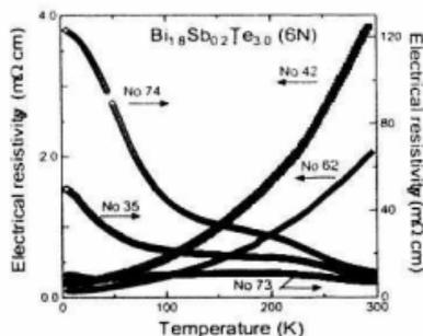
**Fig.2.** Temperature dependence of the electrical resistivity  $\rho$  of various pieces for  $\text{Bi}_{1.8}\text{Sb}_{0.2}\text{Te}_3$  sample.
