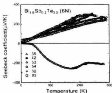
**Fig.1.** Temperature dependence of the Seebeck coefficient  $\alpha$  of various pieces for  $\text{Bi}_{1.8}\text{Sb}_{0.2}\text{Te}_3$  sample.
