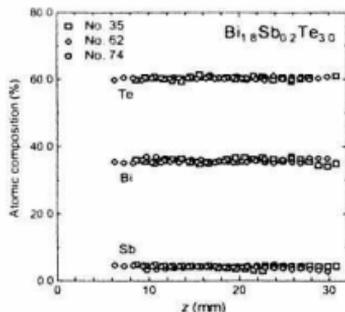
Fig.5. Atomic Bi, Sb and Te composition profiles of  $\text{Bi}_{1.8}\text{Sb}_{0.2}\text{Te}_3$  sample.
