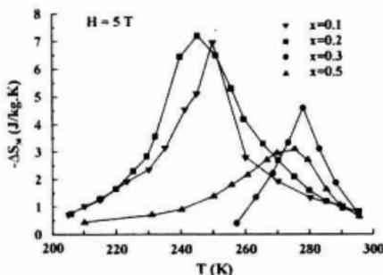
Fig.2. The temperature dependence of  $\Delta S_{\text{mag}}$  of  $\text{La}_{1-x}\text{Ca}_x\text{MnO}_3$
