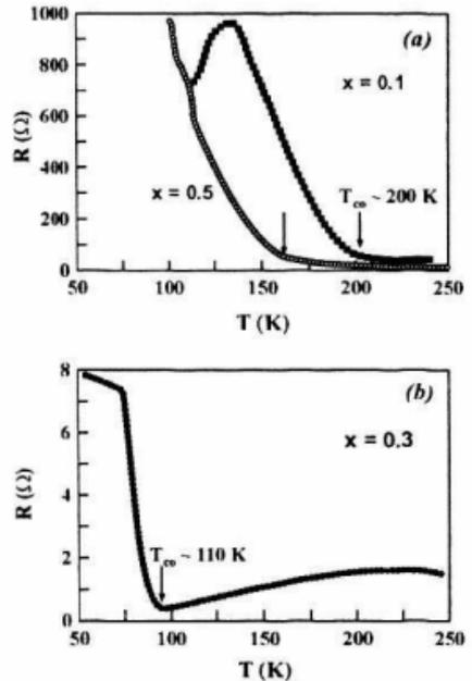
**Fig.3.** Plots of resistivity versus temperature on  $\text{La}_{1-x}\text{Ca}_x\text{MnO}_3$
