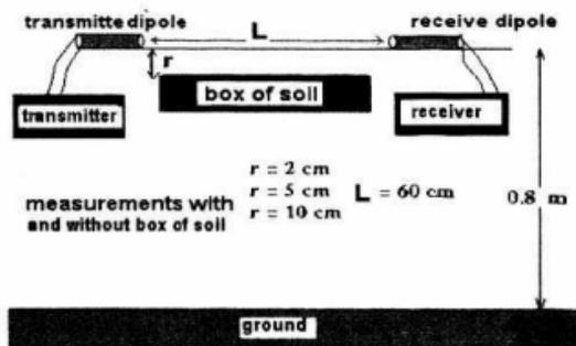
Fig.6. The model of the measurements with dipole-dipole array
