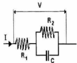
Fig.1. The equivalent circuit for alternating current
