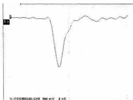
Fig.4. System response time measured by light scattered.
