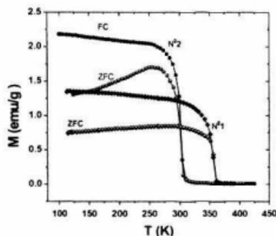
Fig.3. Thermomagnetic field-cooled (FC) and zero-field-cooled (ZFC) curves of samples measured at 20 Oe.
