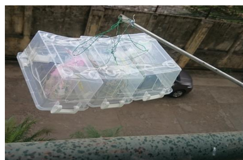
Figure 5. A moss bag hangs on the outdoor to monitor the air metal contents of the site.
