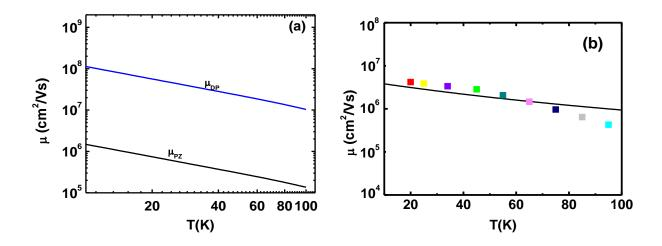
Acoustic-phonon (DP plus PZ coupling) partial mobility dependence on temperature for single-side doped square quantum well.
