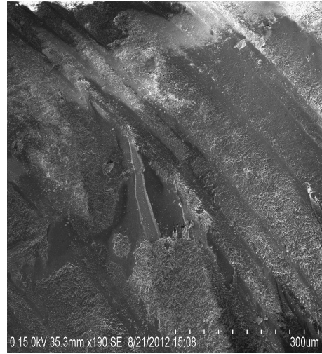
Fig. 4. SEM image of 2Dm composite three-phase material (fibre volume fraction is 25% and particle volume fraction is 3%).
