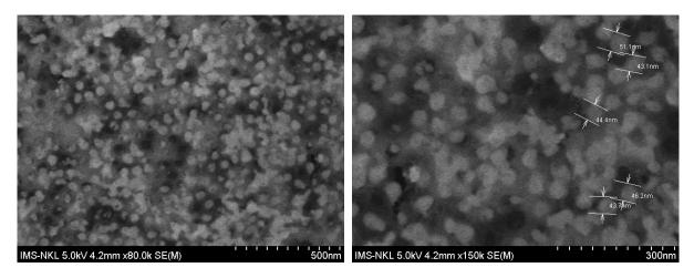
a) b) Figure 2. SEM images of the Cu nanodisk 2D array on the AAO template.
