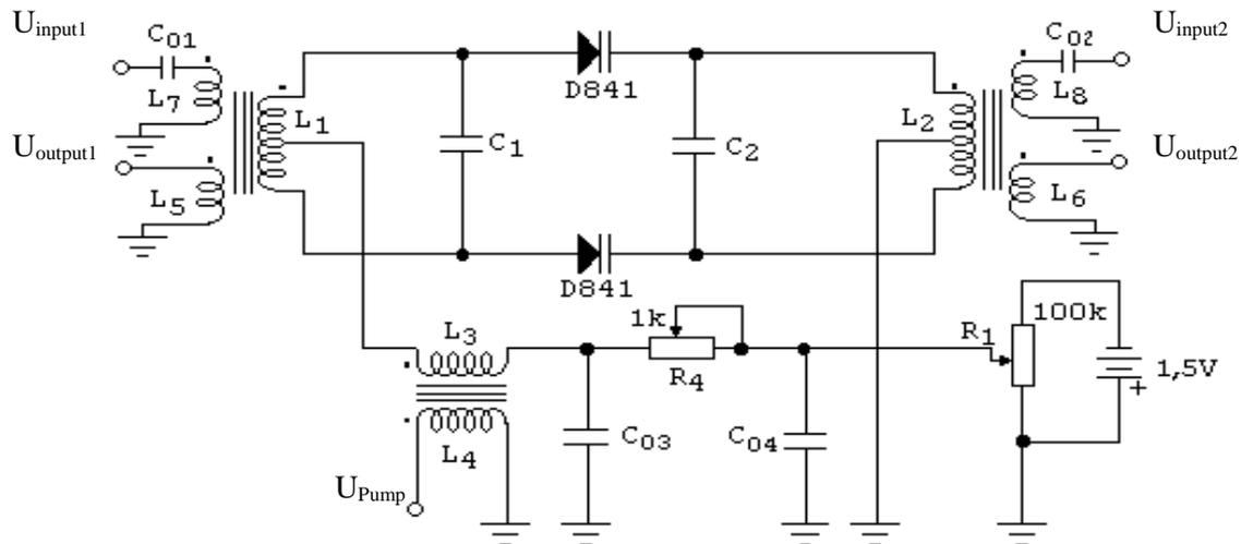
Figure 2. The principle diagram of a dual resonant frame parametric generator.
