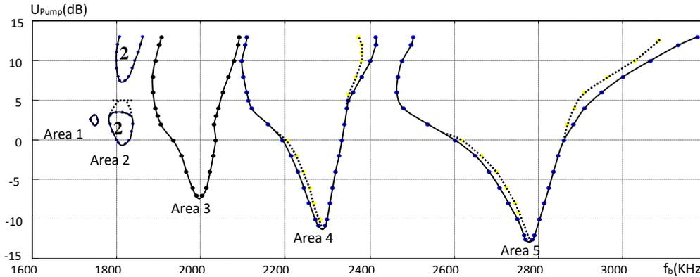
Figure 6. Transmit frequency regions of frame II when changing multiples between two frames ( $\gamma \neq 0$ ).
