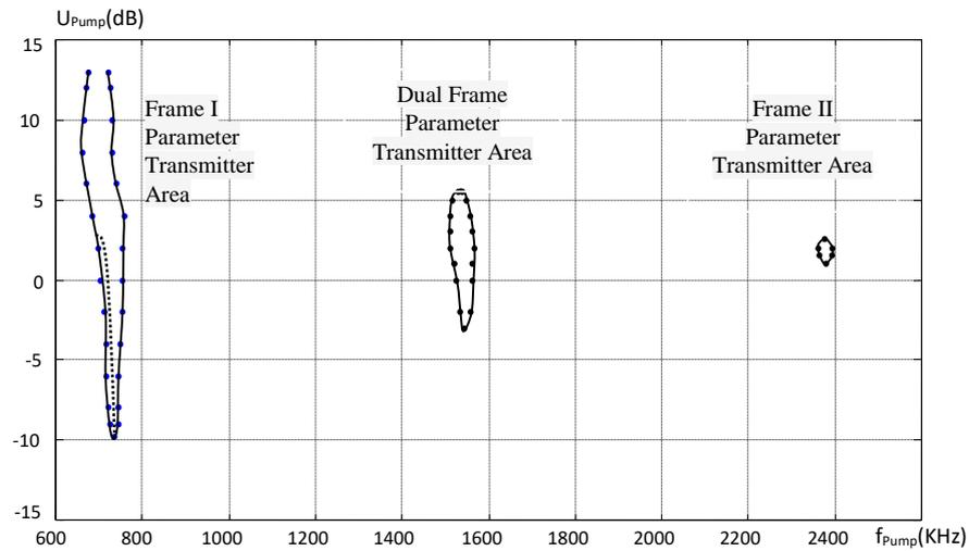
Figure 8. Transmitter zones of a dual resonant frame parameter generator
