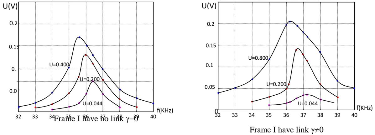
Figure 3. Resonance characteristics of the frame I.
