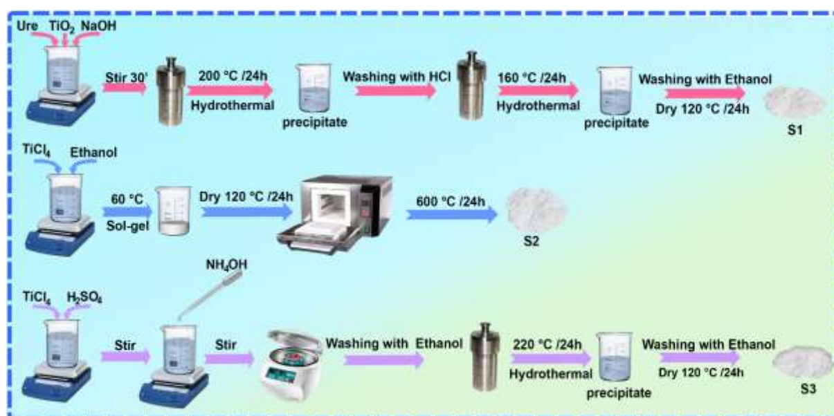
Figure 1. Schematic illustration of synthetic procedure for S1, S2 and S3 samples.
