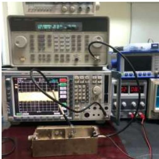
Figure 10. Set of measurement LNA.
