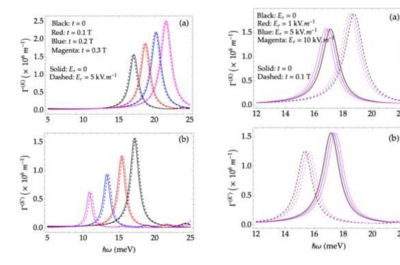
Figure 3. Comparison of absorption spectra between the  $K(\xi=+1)$  (a) and  $K'(\xi=-1)$  (b) valleys as the strain t is varied. In all figures, the colors black, red, blue, and magenta represent strains of 0, 0.1, 0.2 and 0.3 T, respectively. The solid and dashed curves correspond to the cases with and without an in-plane electric field, respectively. In all cases, B=0.5 T, T=4.2 K, and  $n=0\div 2$ .
