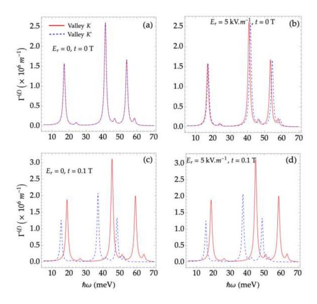
Figure 1. Magneto-optical absorption spectrum for different scenarios of electric field and strain: (a) absence of both electric field and strain; (b) with an electric field of 5 kV.m<sup>-1</sup> and no strain; (c) with a strain of 0.1 T and no electric field; and (d) with both electric field and strain. In all cases, the real magnetic field is B = 0.5 T, the temperature is T = 4.2 K, and the LLs  $n = 0 \div 2$  are considered.
