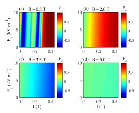
Figure 6. Density plot of the valley polarization versus strain (t) and in-plane electric fied ( $E_r$ ) at the magnetic field of (a) 0.5 T, (b) 2.0 T, (c) 3.5 T, and (d) 5.0 T. Here,  $T=4.2~{\rm K}$  and  $h\omega=40~{\rm meV}$ . Note that all the figures are presented with the same color scale to allow for a comparison of the magnetic field's effect on the valley polarization values.
