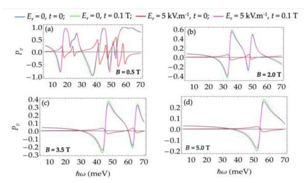
Figure 5. The valley polarization in the absorption coefficient as a function of photon energy for different scenarios of electric field and strain. Figures (a), (b), (c), and (d) correspond to the real external magnetic field of 0.5 T, 2.0 T, 3.5 T, and 5.0 T, respectively. Here, T = 4.2 K.
