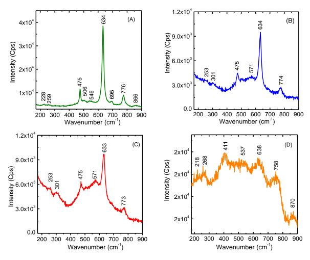
Figure 2. Raman spectra of  $SnO_2$  samples at different annealing temperatures: A- 1100 °C, B- 800 °C, C- 600 °C, D- 400 °C.
