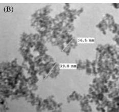
Figure 1. (A) XRD patterns of  $SnO_2$  samples at different annealing temperatures: a- 400 °C, b- 600 °C, c- 800 °C, d- 1100 °C; (B) FESEM image of  $SnO_2$  sample annealed at 600 °C.
