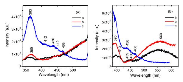
Figure 3. PL spectra under excitation wavelengths of (A) 300 nm and (B) 335 nm of the samples annealed at (a) 400 °C, (b) 800 °C and (c) 1100 °C.
