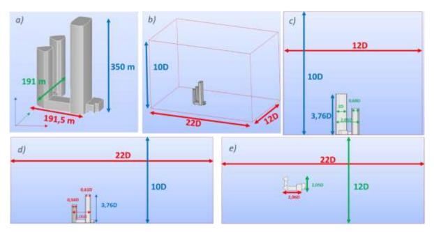
Figure 3. a) Keangnam Landmark Tower's 3D model on SALOME and characteristic lengths; b) 3D representation of the computational domain;
