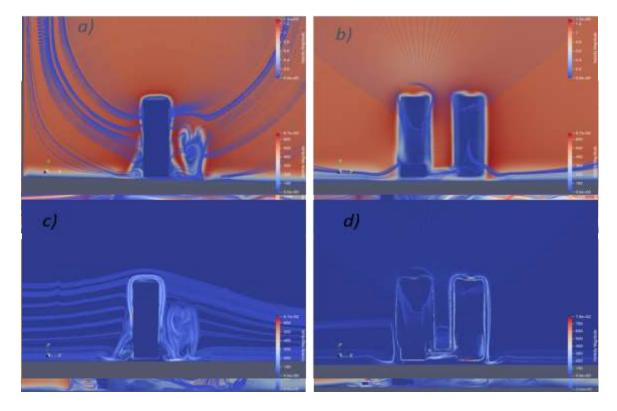
Figure 10. Paraview velocity streamlines on plane X2; b) Paraview velocity streamlines on plane X4; c) Paraview vorticity streamlines on plane X4.
