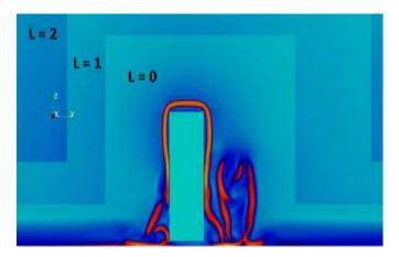
Figure 4. Paraview visualization of the three refinement levels.
