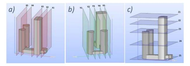
Figure 5. a) Discretization of the 3D model along the X-axis b) Discretization of the 3D model along the Y-axis c) Discretization of the 3D model along the Z-axis.
