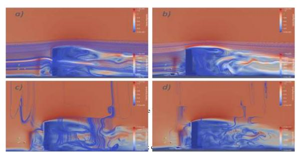
Figure 9. a) Paraview velocity streamlines on plane Y4; b) Paraview velocity streamlines on plane Y5; c) Paraview vorticity streamlines on plane Y4 d) Paraview vorticity streamlines on plane Y5.
