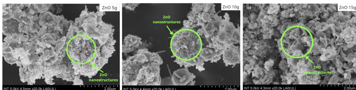
Figure 3. The FE-SEM images of synthesized ZnO nanoparticles with different extract of 5 g, 10 g, and 15 g dried leaves (a-c).
