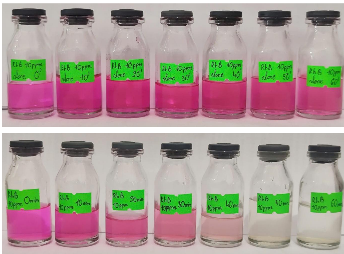
Figure 8. The colour of RhB solution changed under UV light irradiation in the absence (upper image), presence (lower image) of g\text{-C}_3\text{N}_4 nanosheets.
