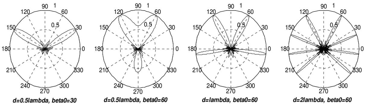
Fig. 7. Radiation pattern while steering for a linear array with different element distance  $d$ .
