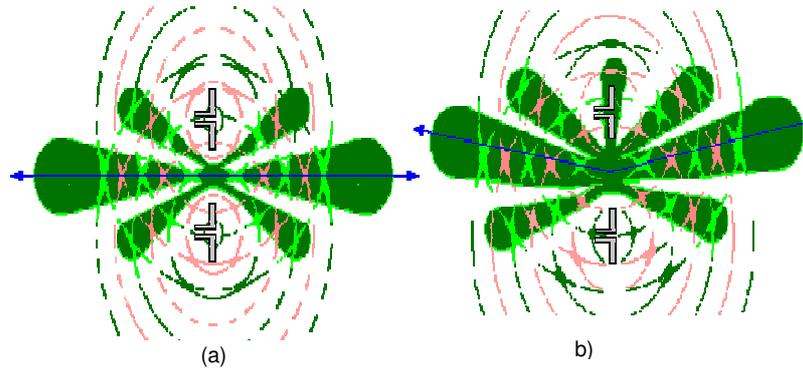
Fig. 3. Two antenna elements. (a) fed with same phase, (b) different phase.
