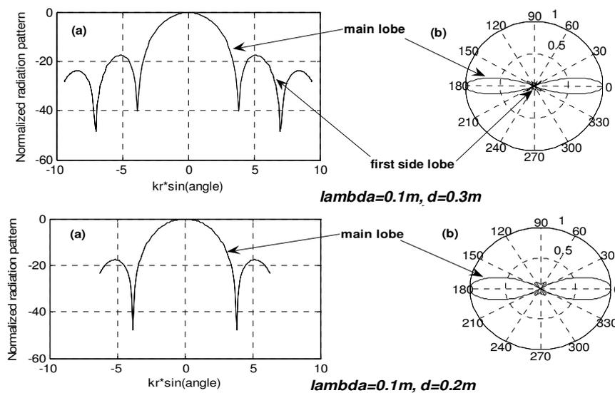
Fig. 5. (a) Circular aperture pattern, (b) Polar plot.
