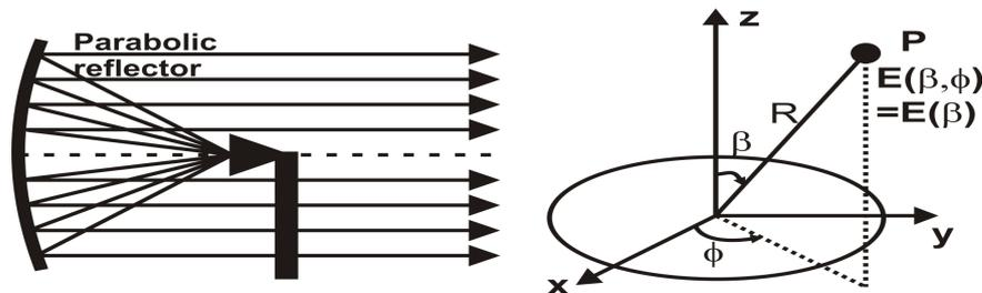
Fig. 2. Parabolic dish antenna model.
