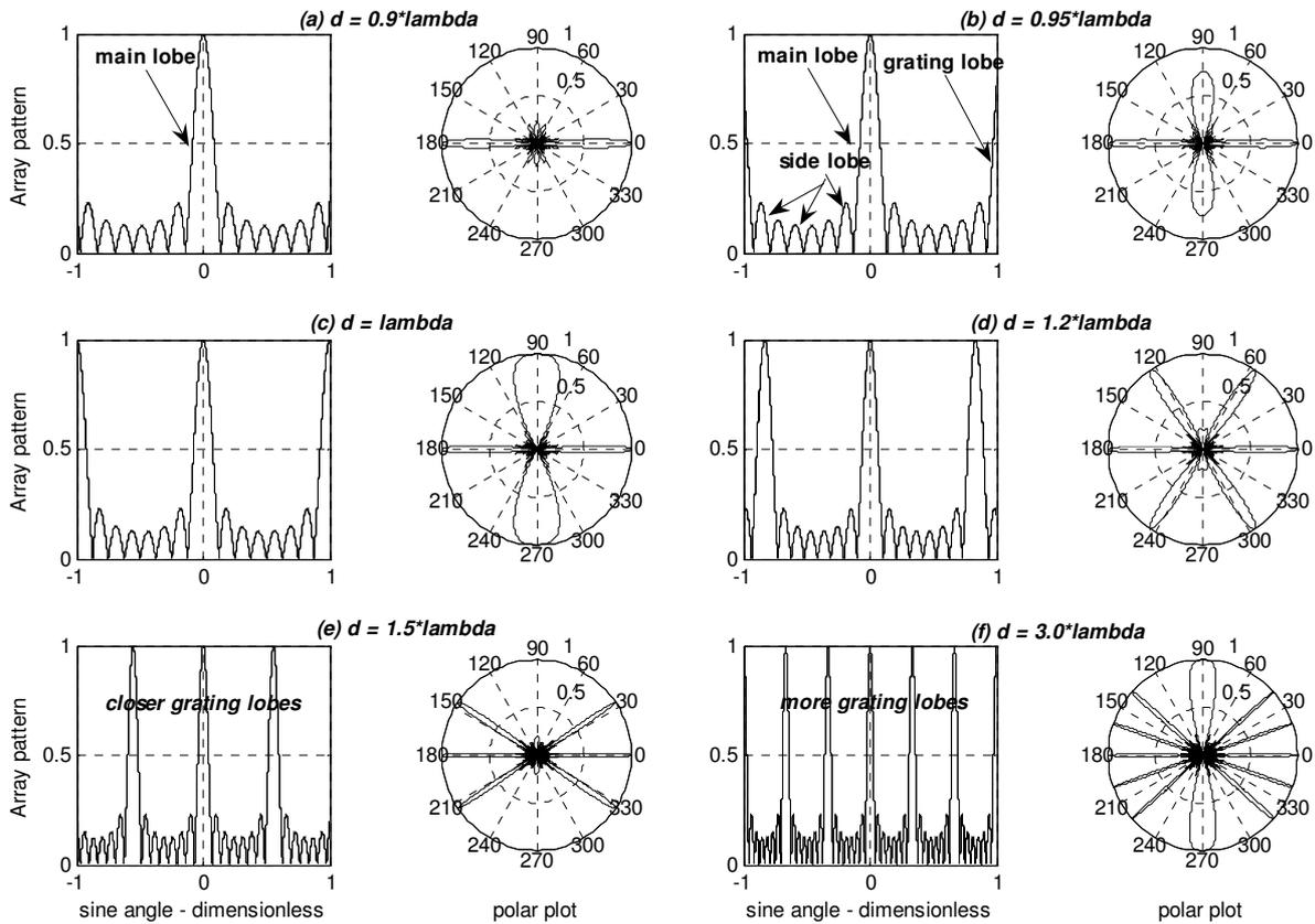
Fig. 6. Radiation pattern for a linear array with different element distance  $d$ .
