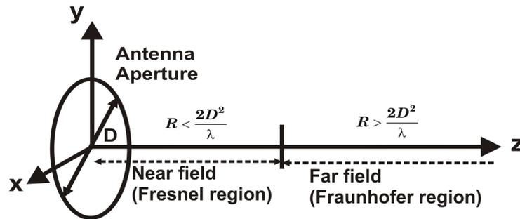
Fig. 1. Near and Far Fields of Antenna.
