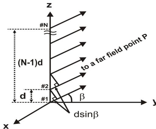
Fig. 4. Uniform linear arrays.
