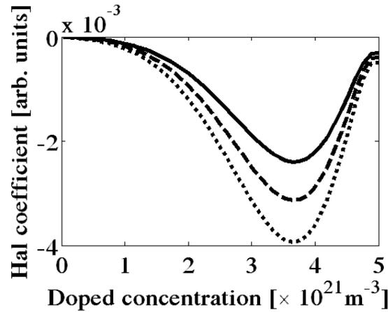
Figure 3. Hall coefficient (arb. Units) as functions of the doped concentration at temperature of 240K (solid line), 270K (dashed line), and 300K (dotted line). Here  $B = 4T$ ,  $E_1 = 5 \times 10^5 Vm^{-1}$ ,  $E_0 = 10^5 Vm^{-1}$ ,  $\omega_p = 4 \times 10^{13} s^{-1}$ ,  $d = 15nm$ , and  $\Omega = 5 \times 10^{13} s^{-1}$ .
