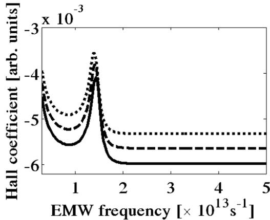
Figure 1. Hall coefficient (arb. Units) as functions of the EMW frequency at different at  $B = 4.00\text{T}$  (solid line),  $B = 4.05\text{T}$  (dashed line), and  $B = 4.10\text{T}$  (dotted line). Here,  $E_1 = 5 \times 10^5 \text{Vm}^{-1}$ ,  $E_0 = 10^5 \text{Vm}^{-1}$ ,  $\omega_p = 4 \times 10^{13} \text{s}^{-1}$ ,  $d = 15\text{nm}$ , and  $T = 270\text{K}$ .
