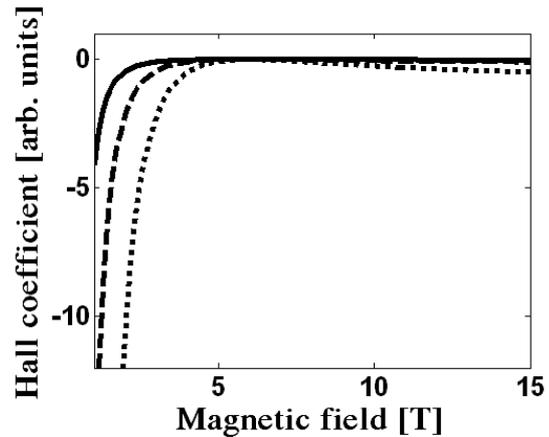
Figure 2. Hall coefficient (arb. Units) as functions of the magnetic field  $B$  at different values of the superlattice period:  $d = 15\text{nm}$  (solid line),  $d = 16\text{nm}$  (dashed line), and  $d = 17\text{nm}$  (dotted line). Here,  $E_1 = 5 \times 10^5 \text{Vm}^{-1}$ ,  $E_0 = 10^5 \text{Vm}^{-1}$ ,  $\omega_p = 4 \times 10^{13} \text{s}^{-1}$ ,  $\Omega = 5 \times 10^{13} \text{s}^{-1}$ , and  $T = 270\text{K}$ .
