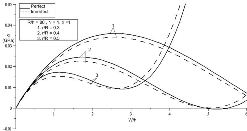
Fig. 6. Effects of radius of base-to-curvature radius ratio  $r/R$  on the nonlinear response of the S-FGM shallow spherical shells.
