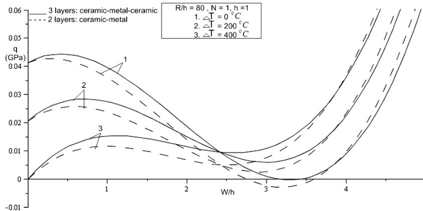
Fig. 7. Effects of temperature field on the nonlinear response of the S-FGM shallow spherical shell under uniform external pressure.
