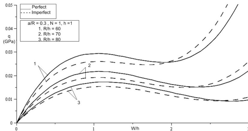
Fig. 5. Effects of curvature radius-to-thickness ratio on the nonlinear response of S-FGM shallow spherical shells
