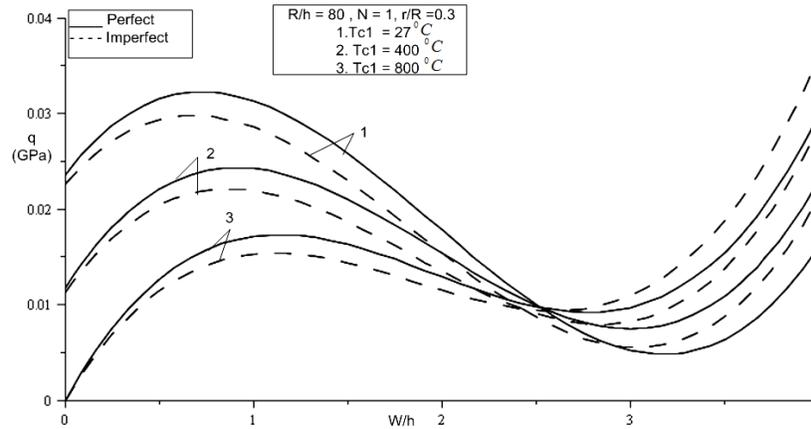
Fig. 8. Effects of temperature gradient on the non-linear response of the S-FGM shallow spherical shell with ceramic-metal-ceramic layers under external pressure.
