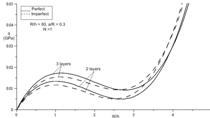
Fig.3. Comparison of the stability of 2 layers (P-FGM) and 3 layers (S-FGM) thin spherical shells.
