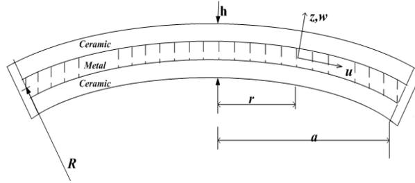
Fig. 1. Configuration and the coordinate system of a S-FGM shallow spherical shell.
