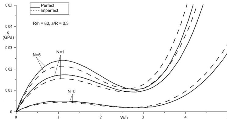
Fig. 4. Effects of volume fraction index N on the nonlinear response of the S-FGM shallow spherical shell.
