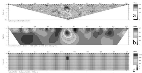
Fig 4. The results of theoretical model with noise environment of 3% and object in depth 1m
