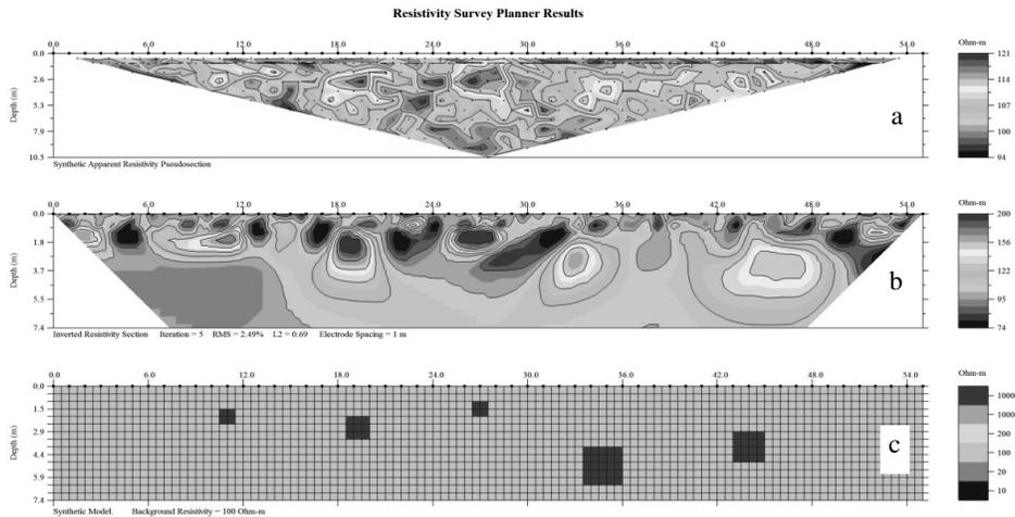
Fig 12. The results of theoretical model with noise environment of 3%
