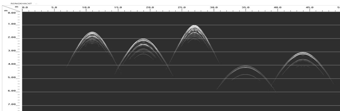
Fig 17. The results of theoretical model with environmental dielectric constant 18 and 5 hollow caves with a dielectric constant of 1, different sizes and located at different depths using the 200 MHz antenna.
