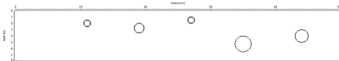
Fig 16. Theoretical hollow cave model with 5 different size objects at different depths used for GPR method.
