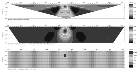
Fig 3. The results of theoretical model with noise environment of 0% and object in depth 1m
