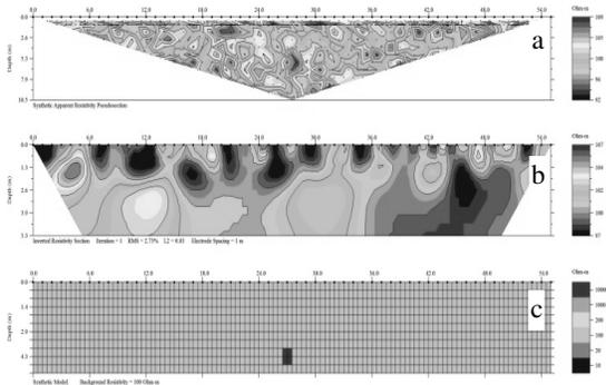
Fig 10. The results of theoretical models with noise environment of 3% and object in depth 4m
