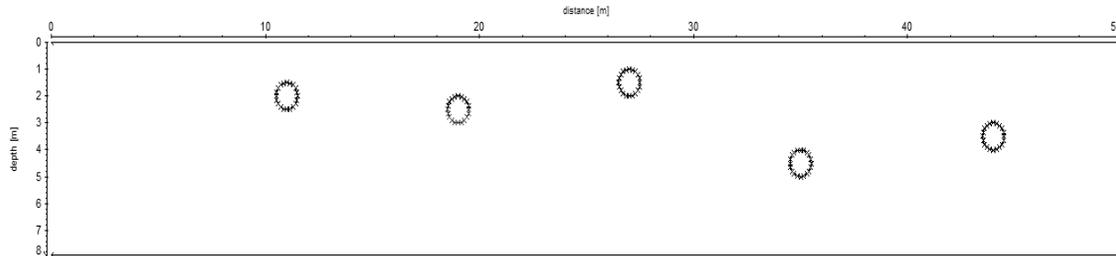
Fig 13. Theoretical hollow cave model with 5 objects of the same size at different depths used for GPR method
