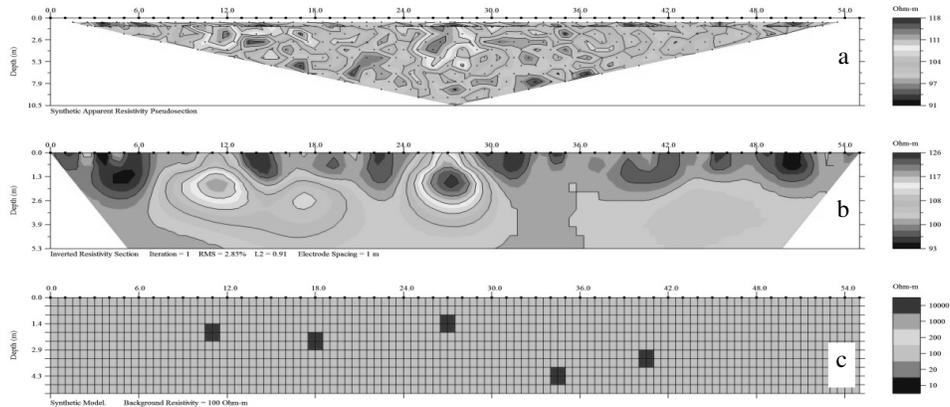
Fig 11. The results of theoretical model with noise environment of 3%
