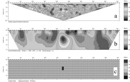
Fig 6. The results of theoretical model with noise environment of 3% and object in depth 2m
