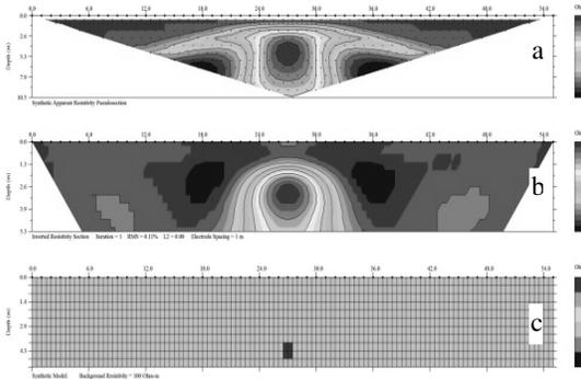
Fig 9. The results of theoretical models with 0% noise environment and object in depth 4m
