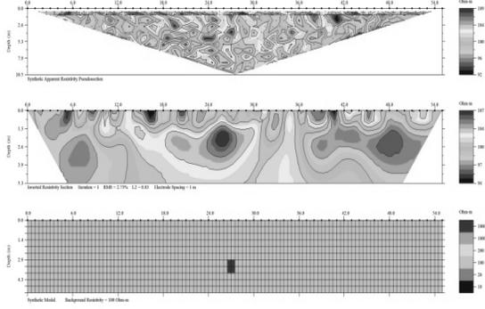
Fig 8. The results of theoretical model with noise environment of 3% and object in depth 3m
