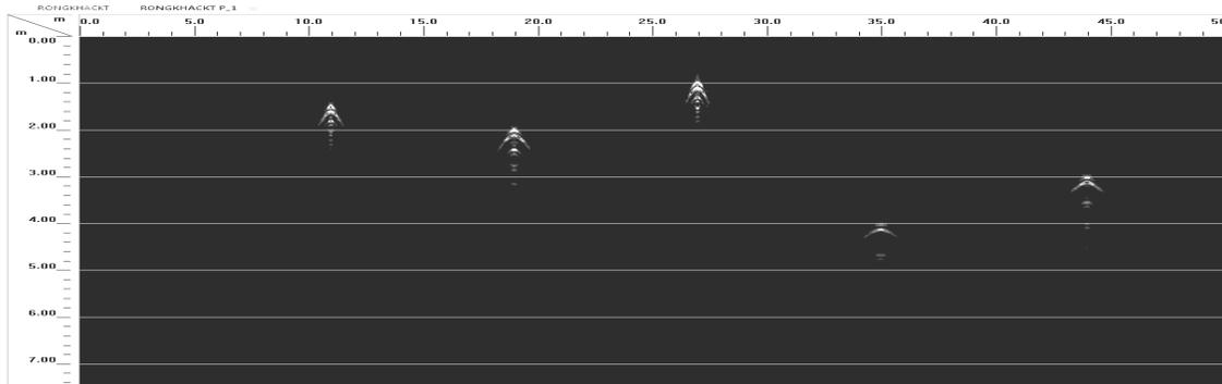
Fig 18. The results of theoretical model with environmental dielectric constant 18 and 5 hollow caves with a dielectric constant of 1, different sizes and located at different depths using the 200 MHz antenna after treatment by allowing movement of Migration.
