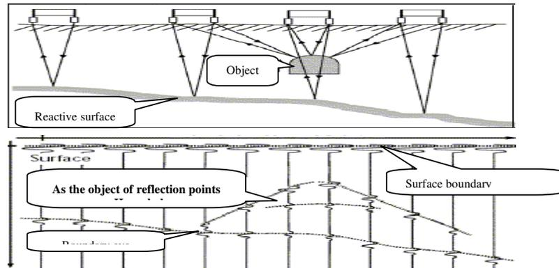
Fig 2. Radar wave diagram on objects.
