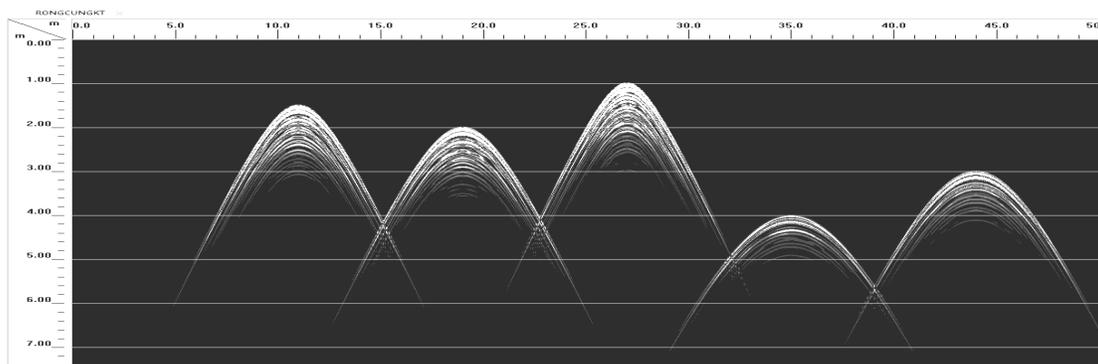
Fig 14. The results of theoretical model with environmental dielectric constant 18 and 5 hollow caves with a dielectric constant of 1, the same size at different depths using 200 MHz antenna.
