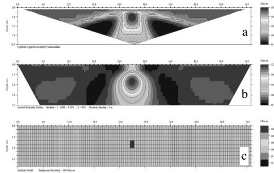
Fig 5. The results of theoretical model with noise environment of 0% and object in depth 2m
