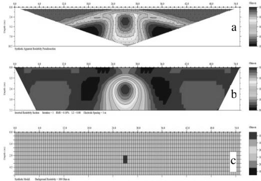
Fig 7. The results of theoretical model with 0% noise environment and object in depth 3m
