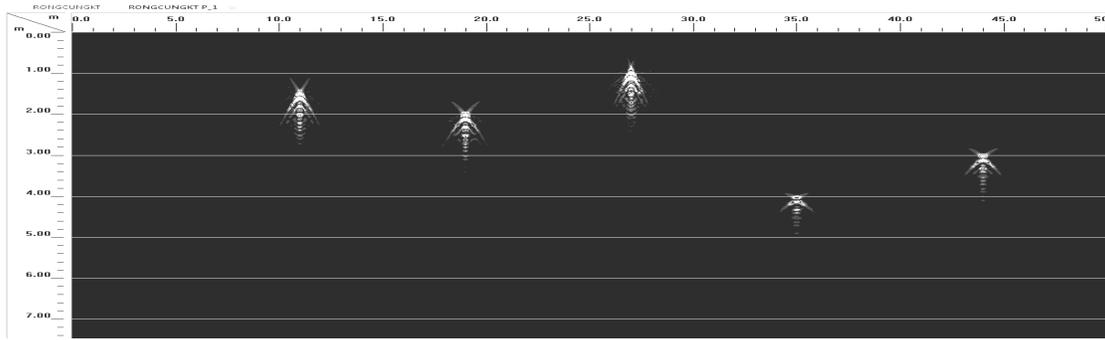
Fig 15. The results of theoretical model with environmental dielectric constant 18 and 5 hollow caves with dielectric constant of 1, the same size and located at different depths using 200 MHz antenna after treatment by allowing movement of Migration.
