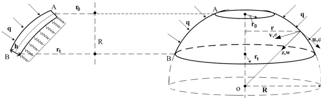
Fig. 1. Configuration of S-FGM annular spherical shell.
