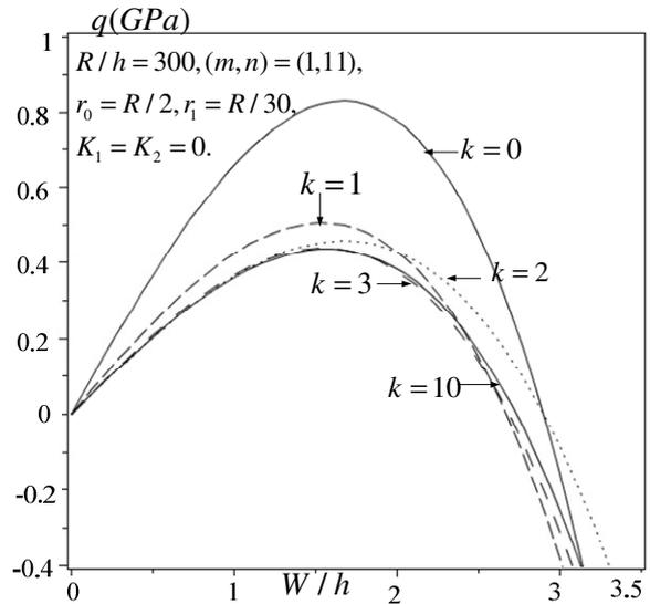
Fig. 3. Effects of volume fraction index  $k$  on the nonlinear response of the S-FGM annular spherical shell.
