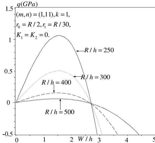
Fig. 4. Effects of curvature radius-thickness ratio on the nonlinear response of the shells under external pressure.
