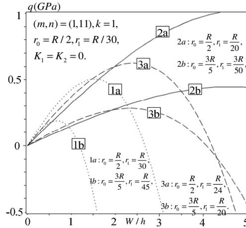
Fig.5. Effects of radius of base-curvature radius ratio  $r_1 / r_0$  on the nonlinear response of the shells.
