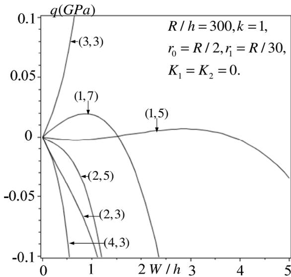
Fig. 2. Effects of mode  $(m, n)$  on the nonlinear response of S-FGM annular spherical shells.
