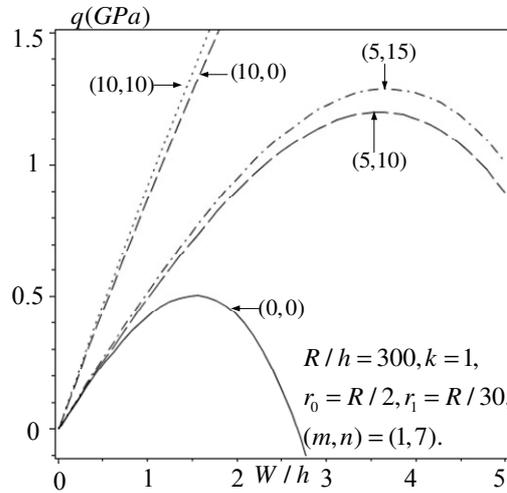
Fig. 6. Effects of the elastic foundations  $(K_1, K_2)$  on the nonlinear response of S-FGM annular spherical shells.
