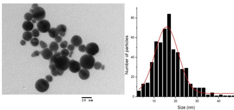
Fig.5. TEM image and size distribution of Au NPs prepared in distilled water.
