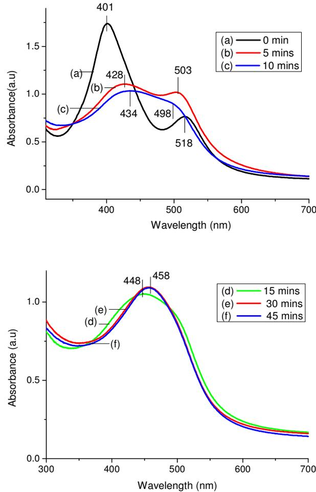
Fig.6. Absorption spectra of a mixture of Au and Ag NPs in distilled water with different irradiation times.
