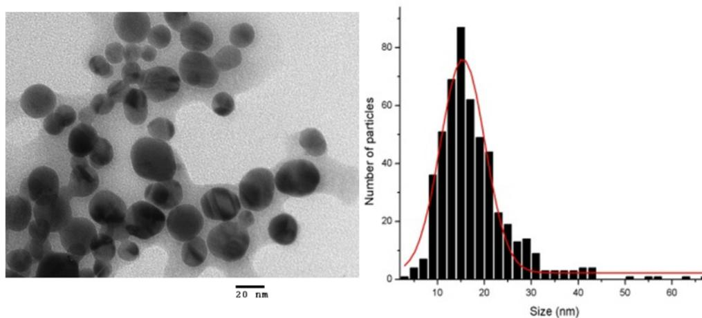
Fig.3. TEM image and size distribution of Ag NPs prepared in distilled water.
