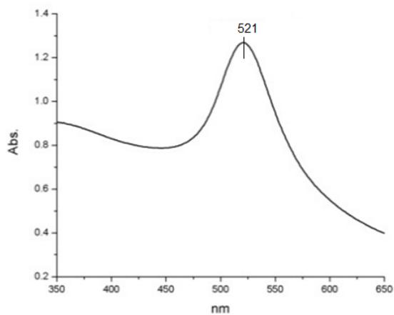
Fig.4. UV-Vis absorption spectrum of colloidal Au NPs.
