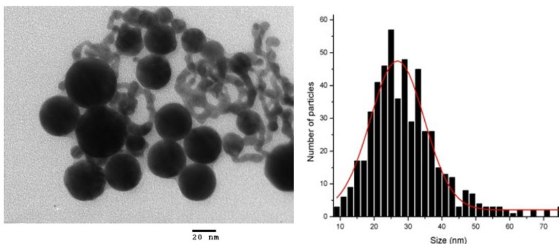
Fig.7. TEM image and size distribution of Au-Ag alloy NPs in distilled water.
