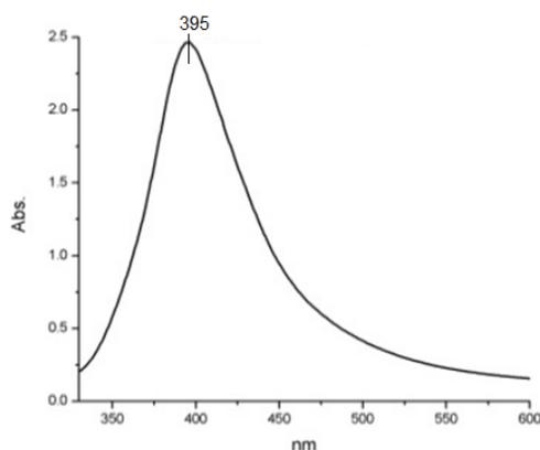
Fig.1. UV-Vis absorption spectrum of colloidal Ag NPs.
