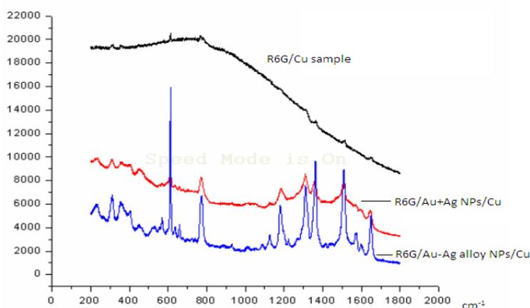
Fig.8. Raman spectra of R6G on SERS substrates.
