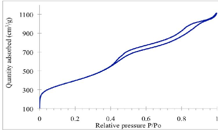
Fig. 2. Nitrogen adsorption/desorption isotherm of the prepared carbon material.
