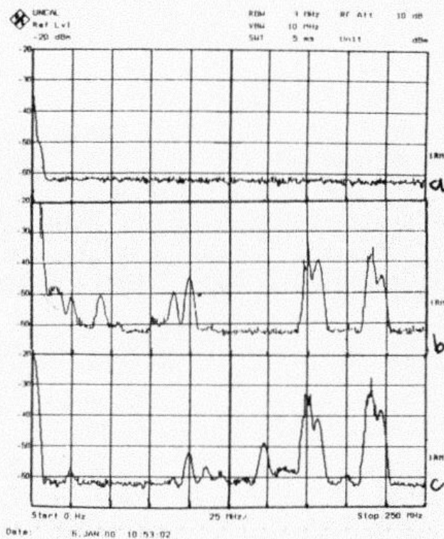
Fig.8: Noise spectrum density: a- Floor noise; b- White noise; c- Noise of sensor
