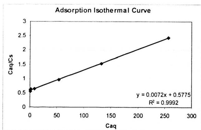
Fig. 5. The Langmuir adsorption Isothermal Curve.
