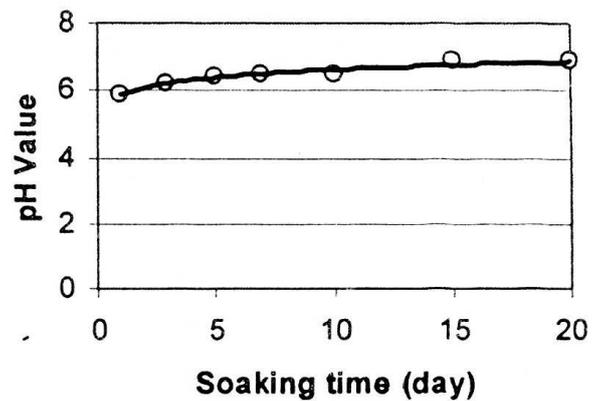
Fig. 3. The variation of pH value of rain water brick soaking.
