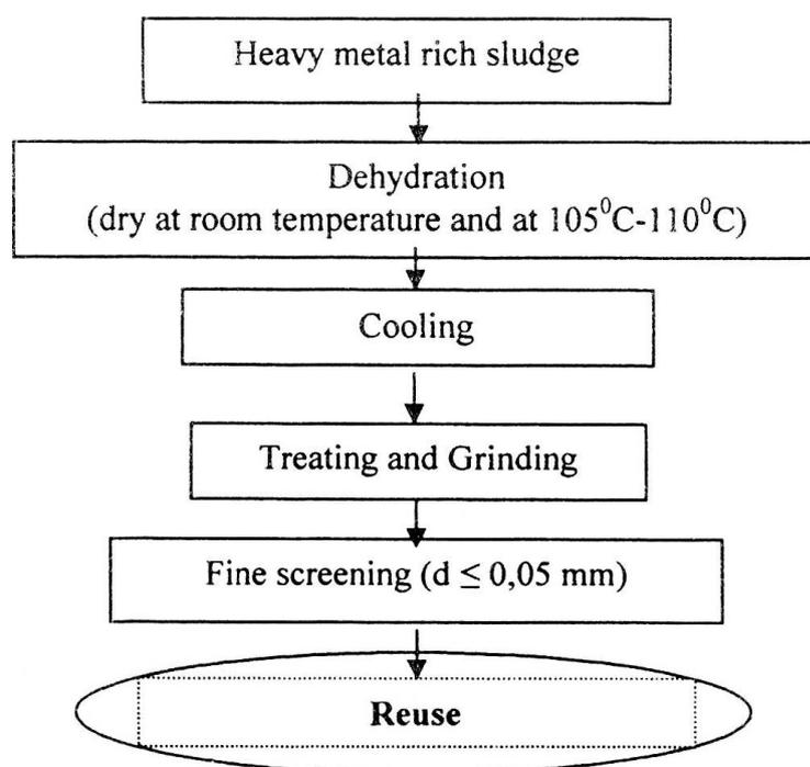
Fig. 1. Diagram of thickened sludge treatment.
